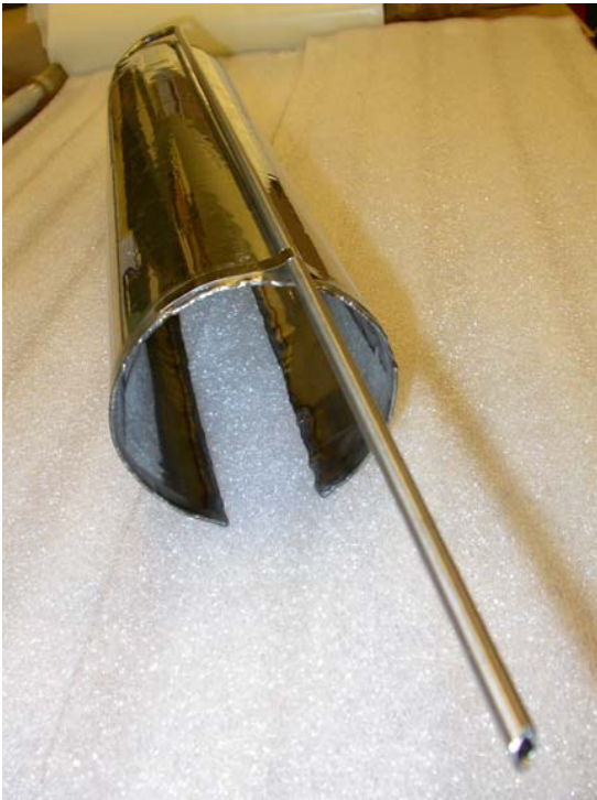
Fig. 5(a) Stainless steel bladder with 0.01" thick wall containing 10 layers of MLI.
