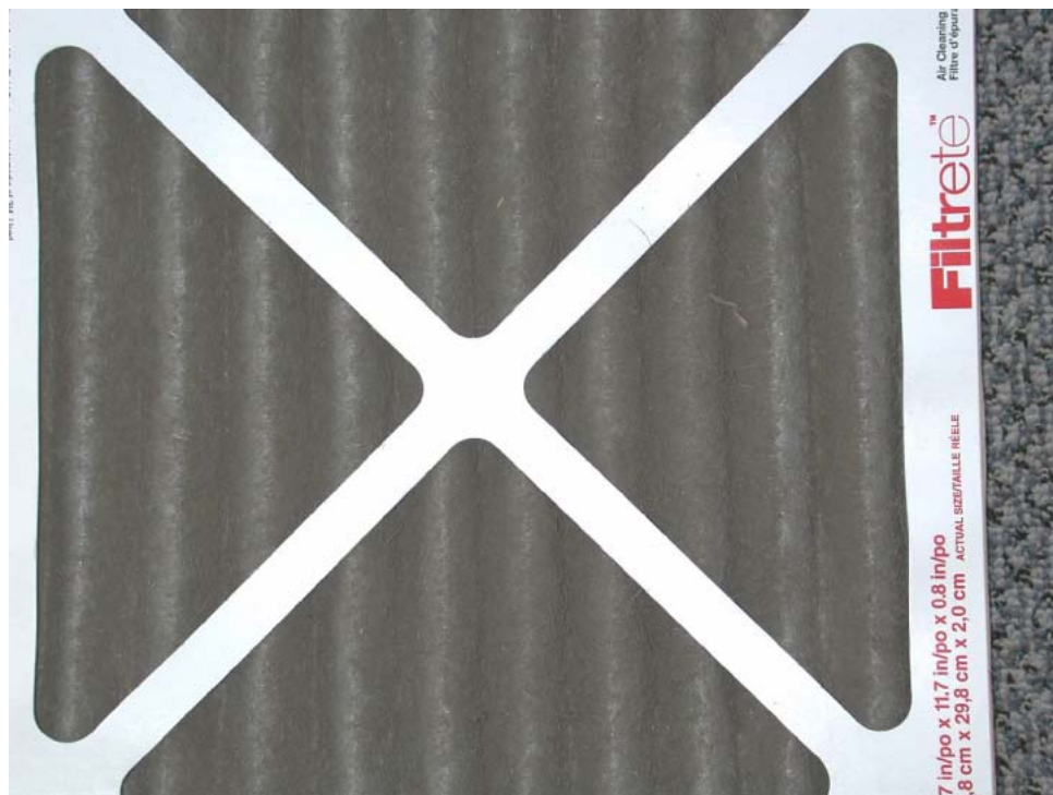
Typical original-design ventilation filter after 90 days – lots of dirt trapped
