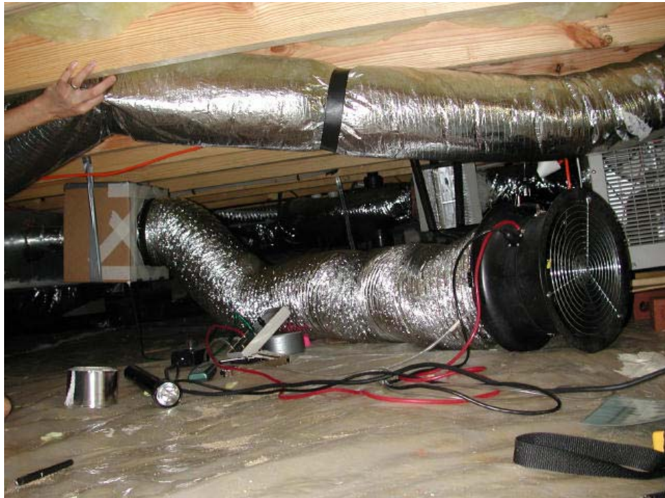
Duct Blaster as powered flow hood to calibrate crawl space supply
