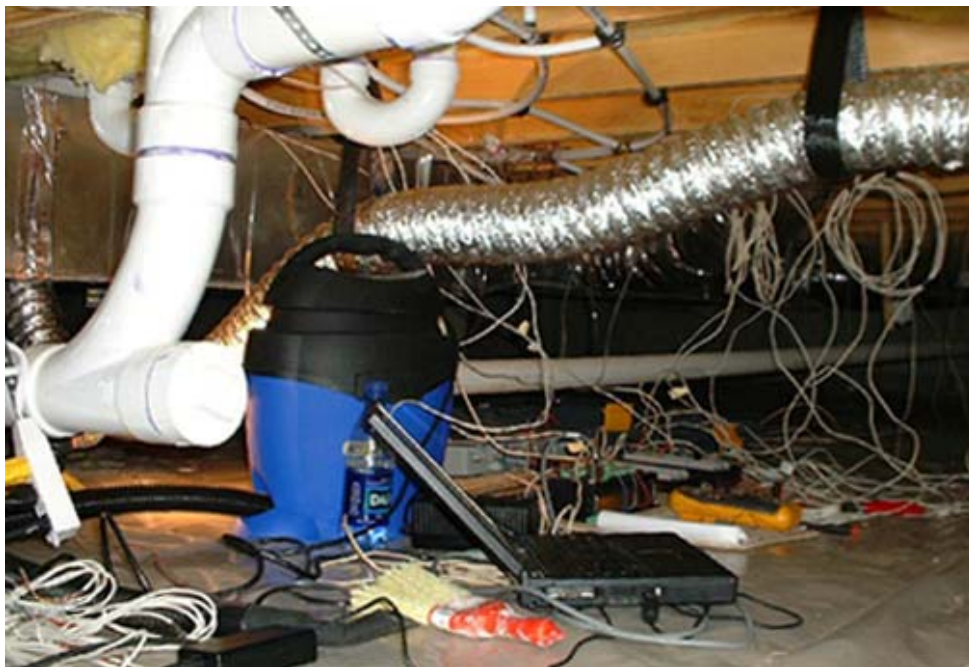
House address 110: Data logger installation - hygrothermal
