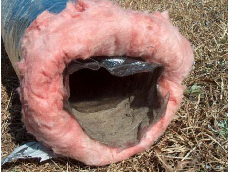
Old ventilation duct prior to filter – substantial soiling
