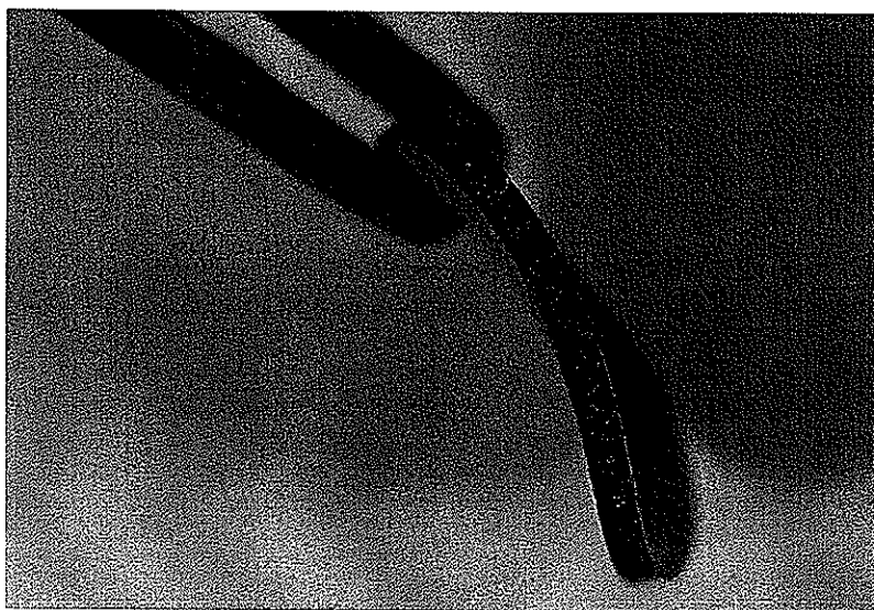
Figure 57. Macroscopic deformation of alloy S20 1 \mu m initial surface finish, cycled 100 times at 500°C/min from 760 (1 hour hold) to 1150°C (1hour hold)
