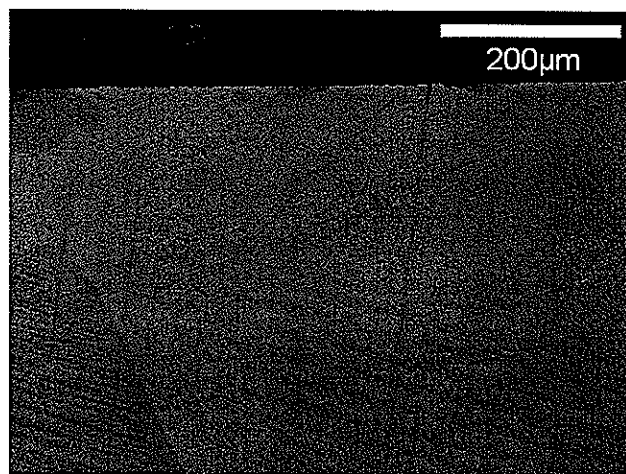
Figure 68. Ni-40Al-15Pt with 1 \mu m initial surface finish, held at 1150°C for 1 hour then cooled at 500°C/min to room temperature
