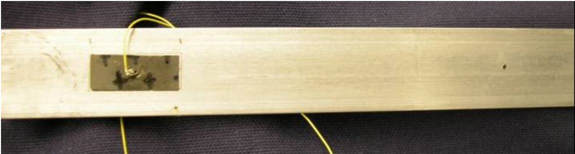
Figure 2.5. Experimental specimens with sensor, and structural flaw. (a) Brass tube; (b) Aluminum plate; (c) Partial beam.
