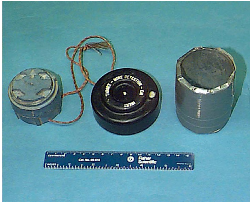
Figure 2: Objects used in the Preliminary Experiments (the can of PlayDough is not shown). On the left is a M14 mine (inert), in the center is a nondescript Mine Detection Target (MDT), and on the right is a nipple covered in duct tape.
