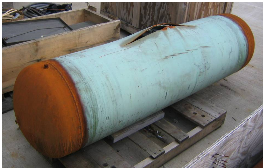
Figure 113 - Pipe With Carbon Fiber-Reinforced Liner (Design 1) Repair After Burst Test
