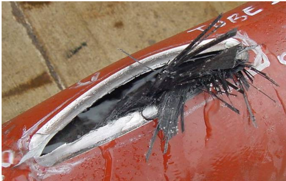
Figure 97 - Pipe Section with Long, Shallow Simulated Corrosion Damage – With Liner – Following Hydrostatic Pressure Test
