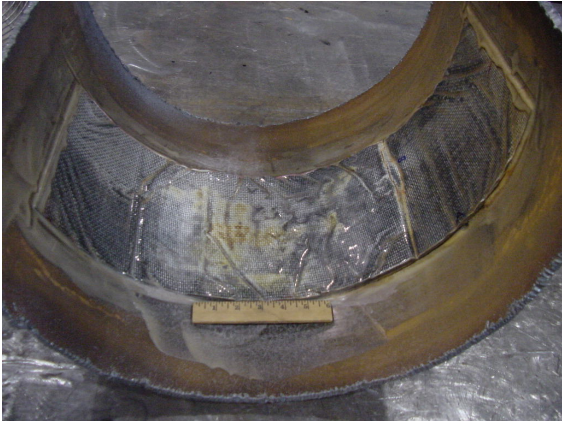
Figure 33 - Pressure Bandage Carbon Fiber-Reinforced Patch (Design 2)
