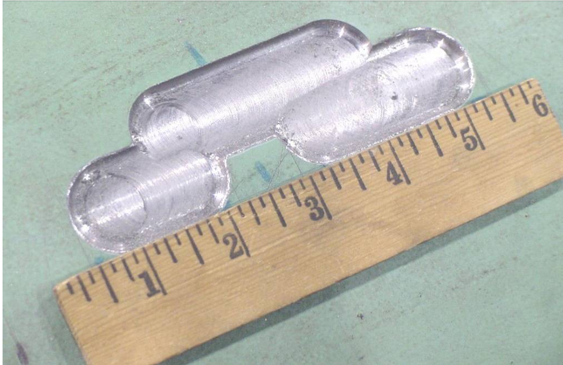
Figure 110 - Selected Configuration of Simulated Damage for 508 mm (20 in.) Diameter Pipe Sections
