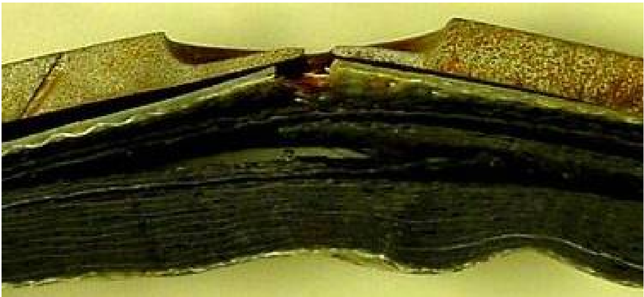
Figure 142 - Disbondment Between Pipe and Patch 2 at Pipe Failure Site
