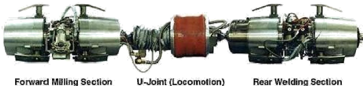
Figure 5 - Welding and Inspection Steam Operations Robot (WISOR)
