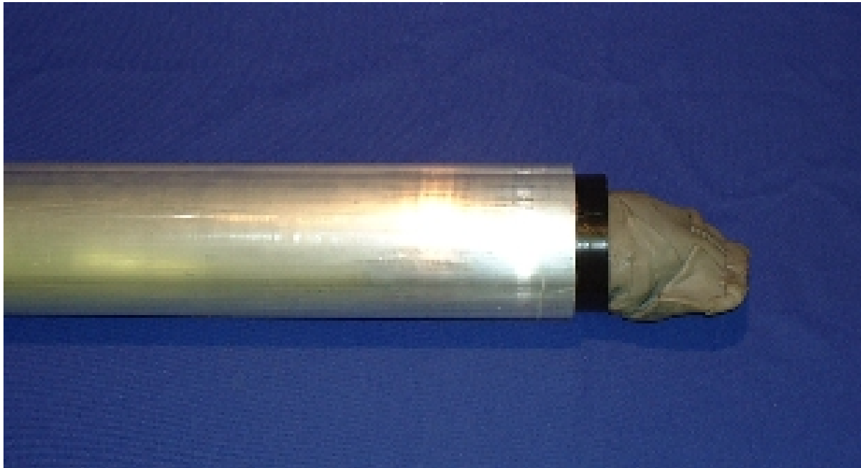
Figure 14 - Silicon Rubber Bag Inserted into Liner
