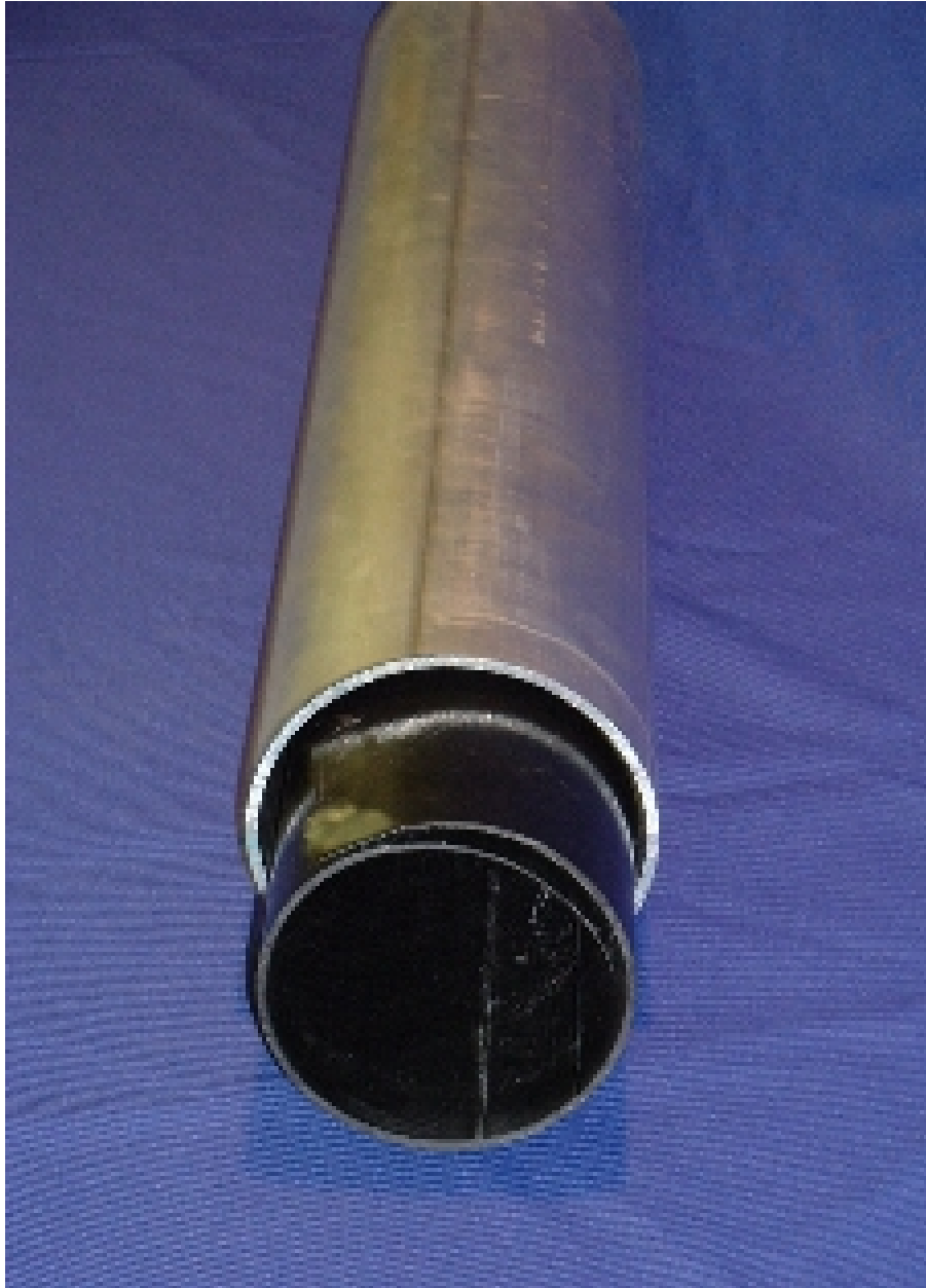
Figure 13 - Insertion of Liner into 114.3 mm (4.5 in.) Diameter Pipe
