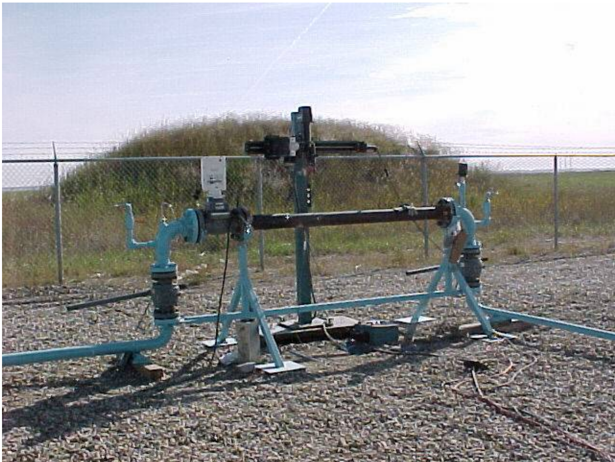
Figure 122 - Experimental Set-Up for Welding onto Thin-Wall Pipe containing Pressurized Methane Gas
