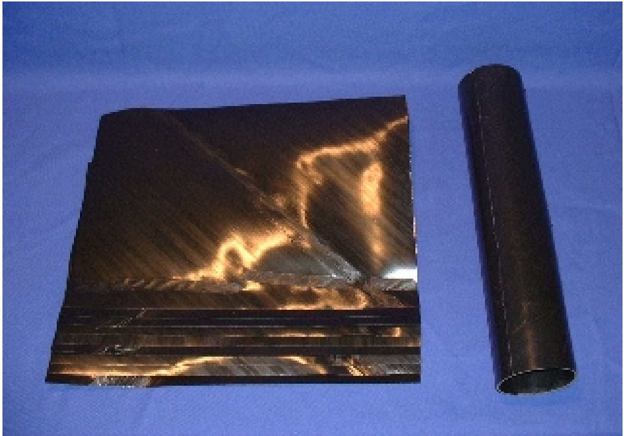
Figure 12 - Lay-Up and Forming of Fiber-Reinforced Composite Liner
