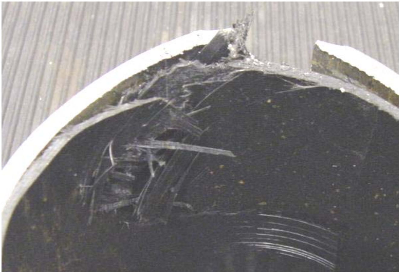
Figure 101 - Pipe Sample Containing Round-Bottom Longitudinal Slot Showing Rupture of Liner Material
