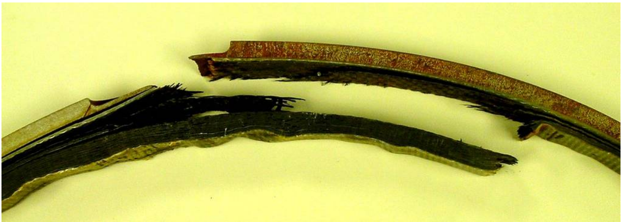
Figure 141 - Failure of Pipe and Composite Repair
