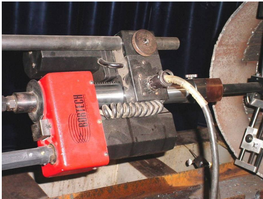
Figure 44 - Bortech Motion Mechanism for Continuous Spiral Deposition
