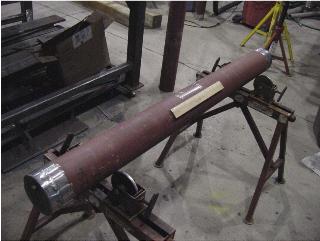
Figure 19 - 114.3 mm (4.5 in.) Diameter Pipe Section with Simulated Corrosion Damage and Welded End Caps
