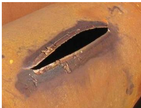
Figure 146 - Patch Design 3 Repair of Long-Shallow Damage after Burst Test
