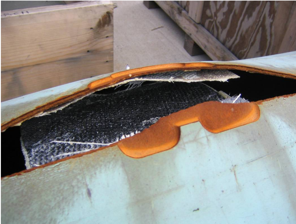
Figure 114 - Failure Initiation Site For Burst Tested Pipe With Carbon Fiber-Reinforced Liner Repair (Design 1)
