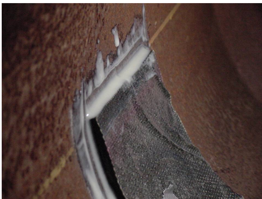
Figure 32 - Adhesive Fillet Around Repair Patch (Design 1)
