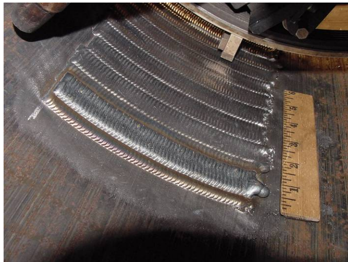
Figure 64 - First Pass of Second Layer of Deposited Weld Metal on Inside Pipe Diameter
