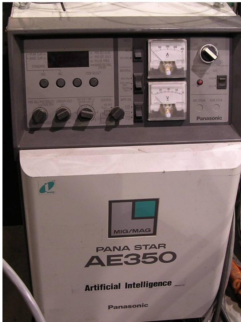
Figure 52 - Panasonic AE 350 Power Supply with Pulse Short-Circuit Metal Transfer Control
