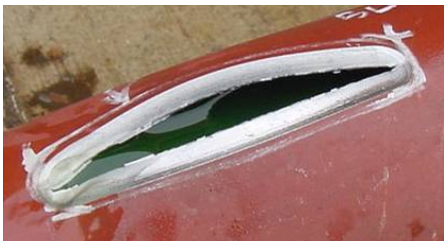
Figure 96 - Pipe Section with Long, Shallow Simulated Corrosion Damage – Without Liner - Following Hydrostatic Pressure Test
