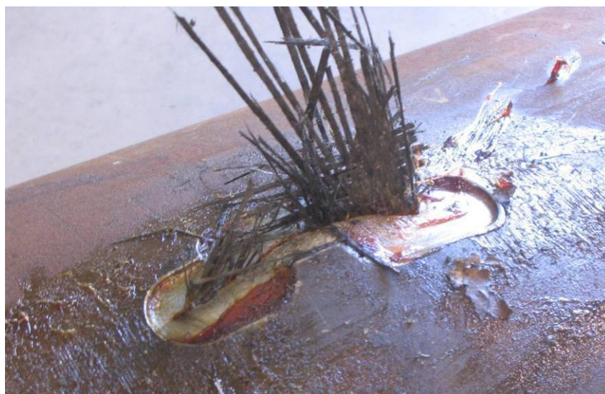
Figure 145 - Failure of Pipe Section with Patch Design 3
