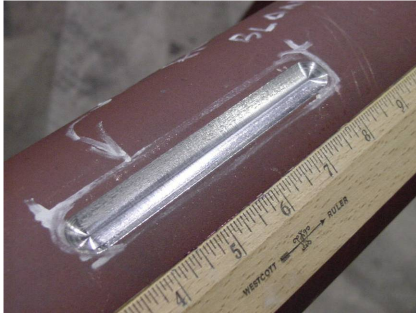
Figure 17 - Long, Shallow Simulated Corrosion Damage
