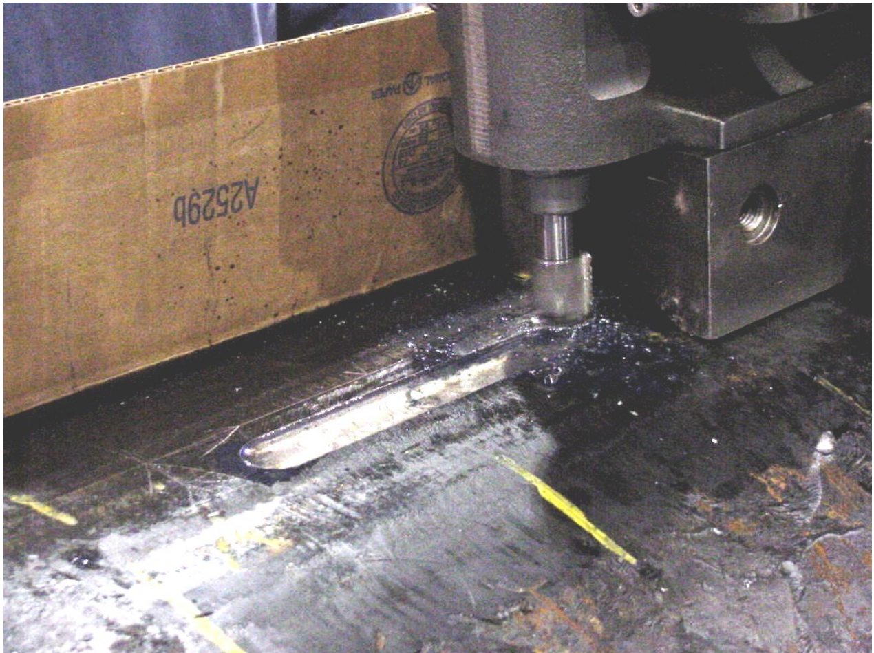
Figure 53 - Milling Machine Set-Up Used to Simulate Corrosion on Pipe Sections
