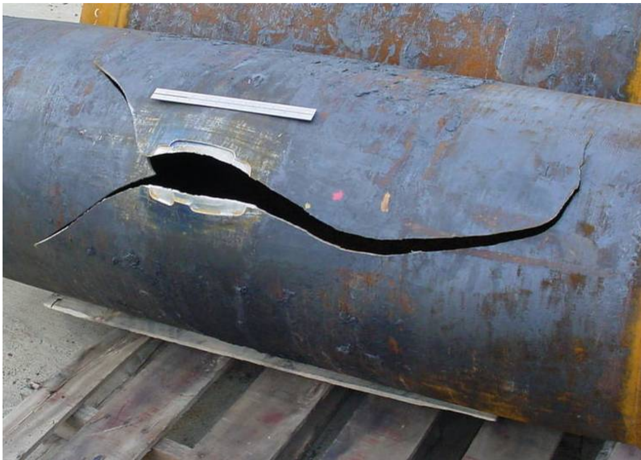
Figure 139 - Hydrostatic Burst Specimen of 558.8 mm (22 in.) With Un-Repaired Damage
