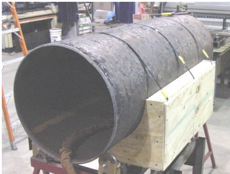
Figure 58 - Orientation of Pipe Section with Dirt Box for Weld Deposition Repair
