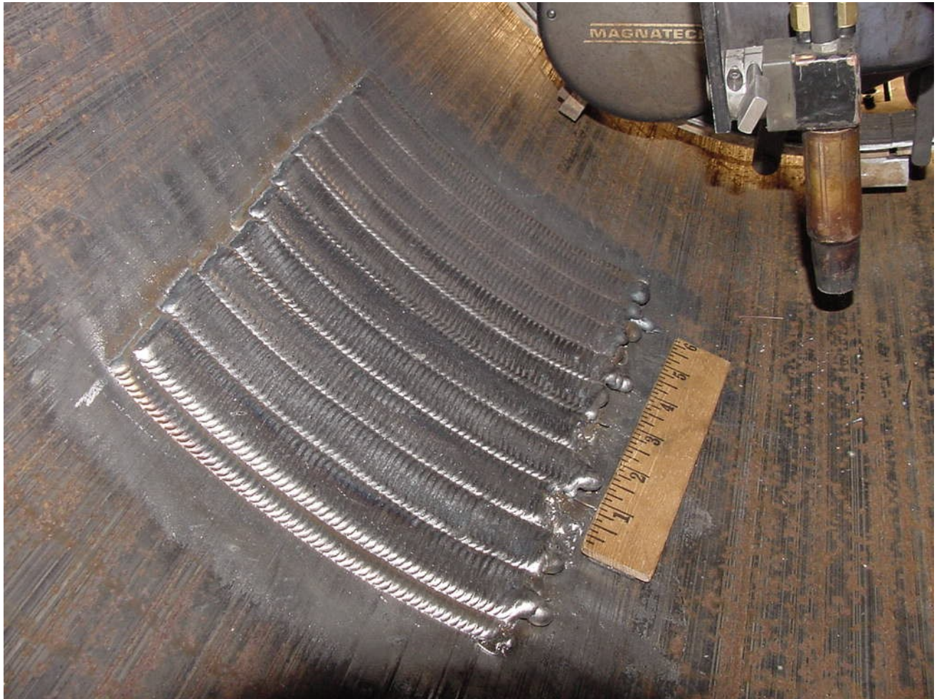
Figure 65 - Finished Second Layer of Deposited Weld Metal on Inside Pipe Diameter
