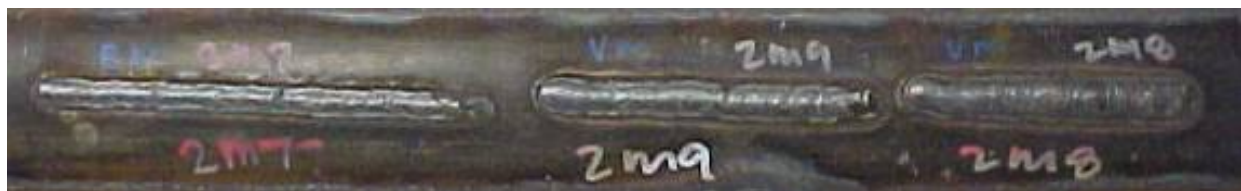
Figure 123 - External Appearance of Welds Made on 3.2 mm (0.125 in.) Thick Pipe with Methane Gas at 4.5 mPa (650 psi) and 6.1 m/sec (19.9 ft/sec) Flow Rate
