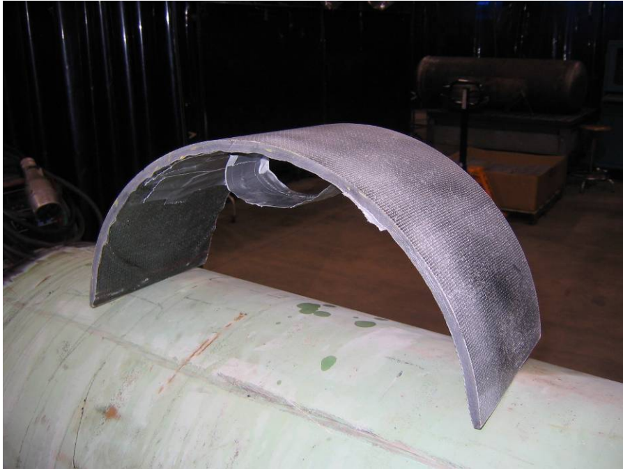
Figure 27 - Completed Repair Patch (Design 1) with Grit-Blasted Outer Diameter
