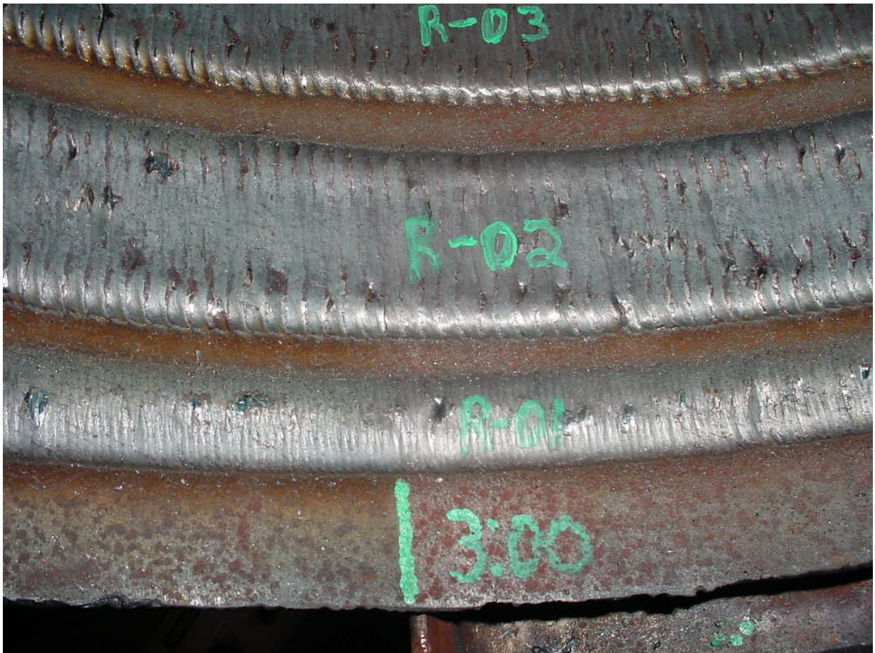
Figure 107 - Tests R-01 and R-02 at 3:00 Showing Steady-State Bead Shape
