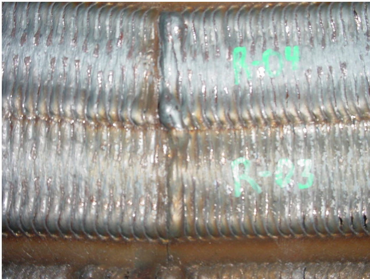
Figure 106 - Tests R-03 and R-04 at 12:00 Showing Better Stop-Start Overlap.
