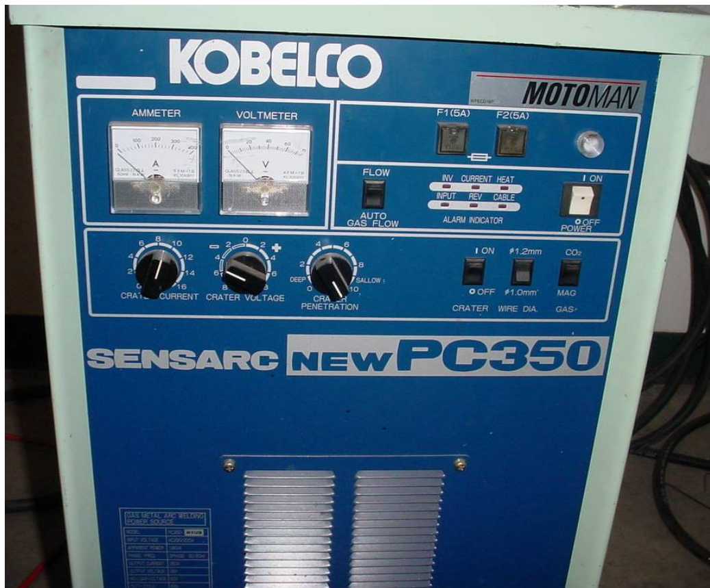
Figure 49 - Kobelco PC-350 Variable Polarity Fuzzy Logic Power Supply
