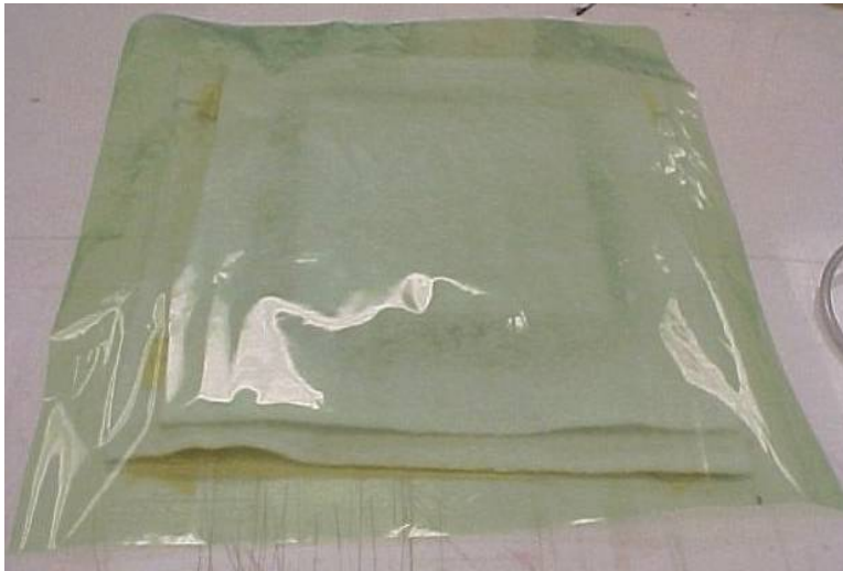
Figure 38 - Vacuum Bag Added Over Sealer Tape
