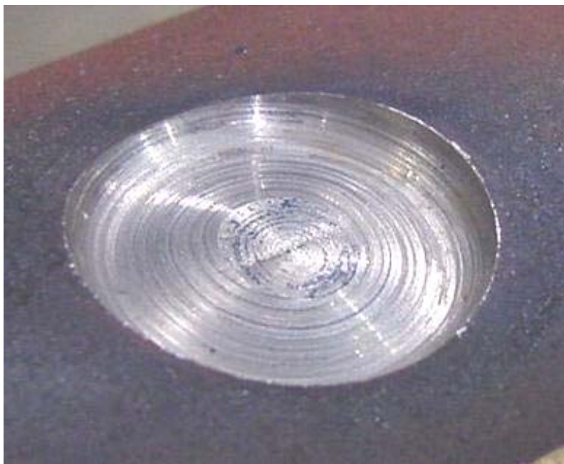
Figure 99 - Pipe Section with Short, Deep Simulated Corrosion Damage – With Liner – Following Hydrostatic Pressure Test
