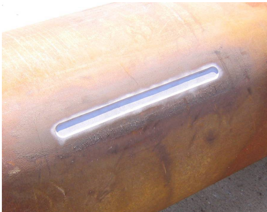
Figure 41 - Long-Shallow Simulated Corrosion
