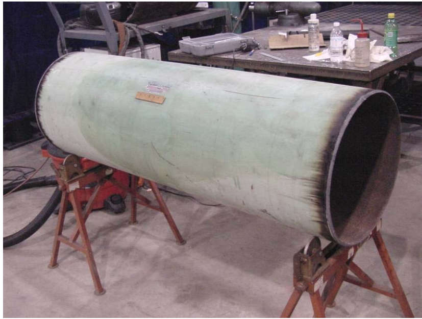
Figure 20 - Pipe Section Used for Test of Carbon Fiber Patch Design No. 1
