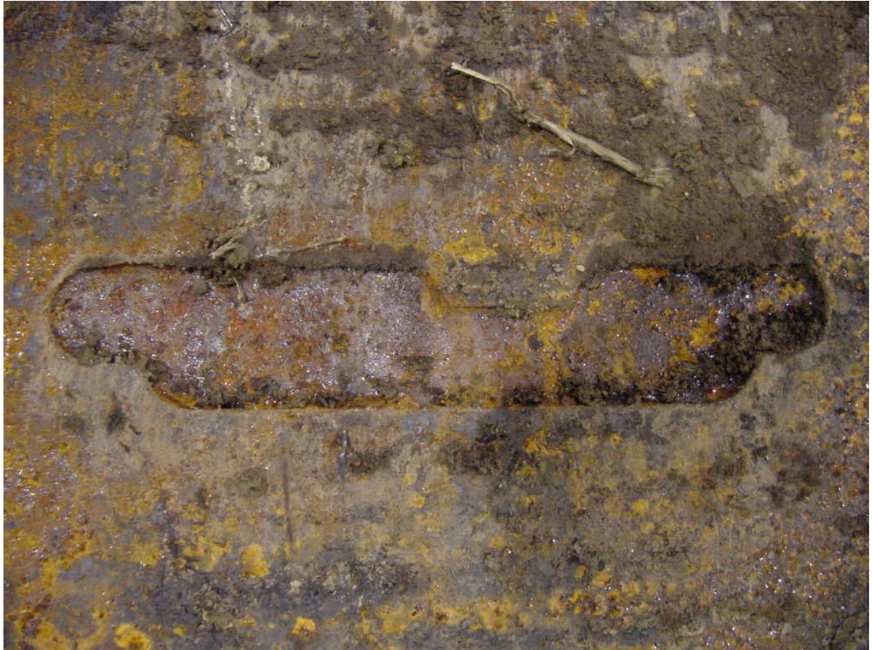
Figure 117 - Simulated Corrosion on Outside of Pipe After Internal Weld Deposition Repair
