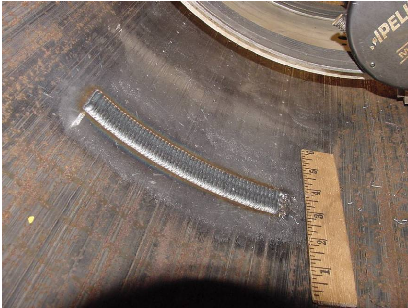
Figure 60 - First Pass of First Layer of Deposited Weld Metal on Inside Pipe Diameter
