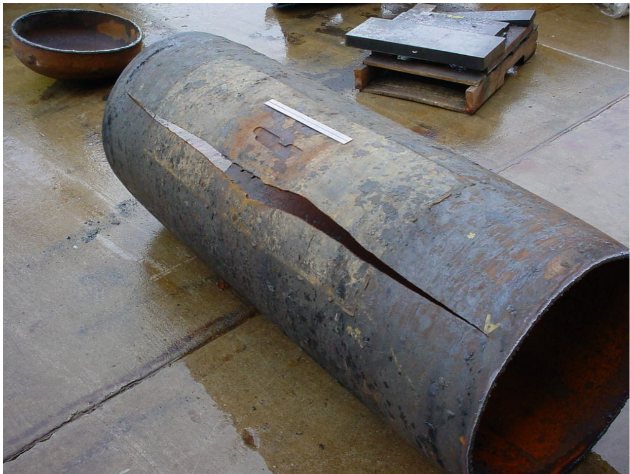
Figure 121 - Pipe Section with Internal Weld Deposition Repair After Hydrostatic Burst Test
