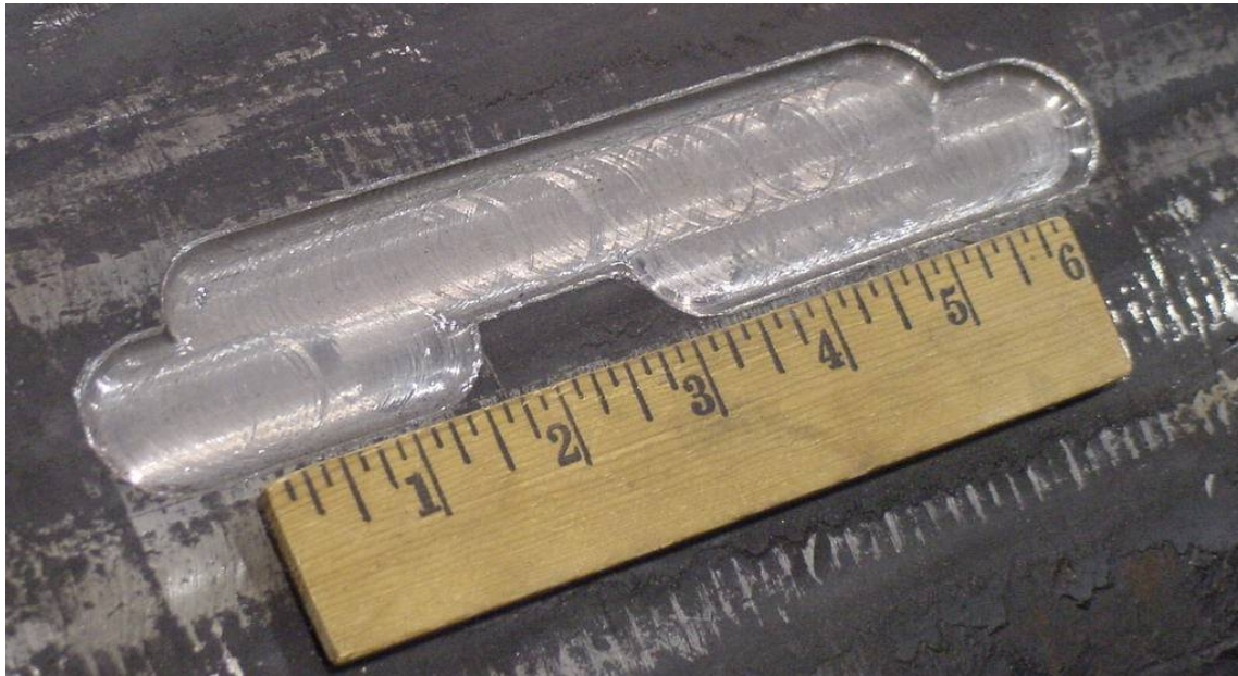
Figure 56 - Magnified View of Simulated Corrosion on 558.80 mm (22 in.) Pipe
