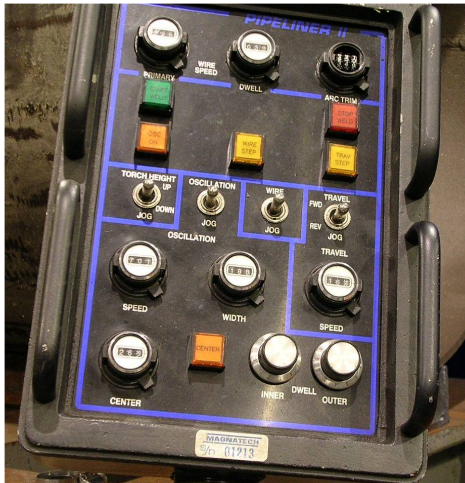
Figure 51 - Magnatech Control Pendant Showing Control Parameters
