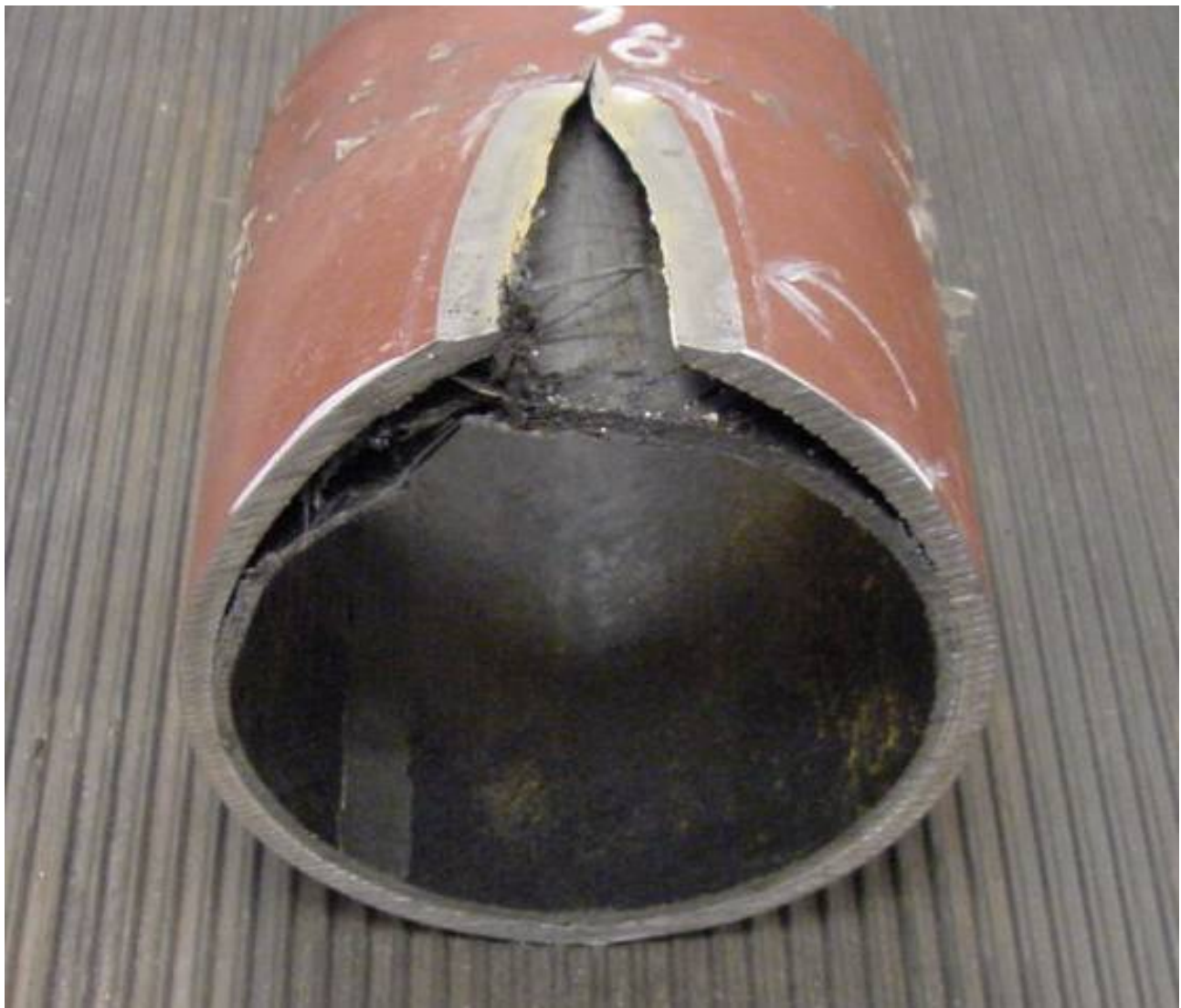
Figure 100 - Water-Jet Cut Section through Pipe Sample Containing Round-Bottom Longitudinal Slot with Liner Installed
