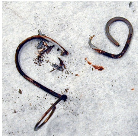
Figure A.11: Wire 4 after Shattering in Vessel
