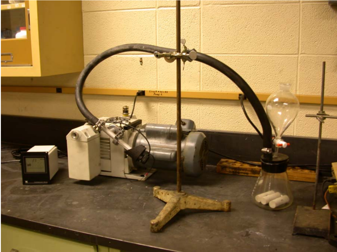
Figure 18: The experimental set-up for porosity measurement.
