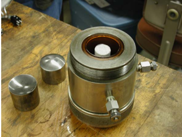
Figure 27: Packing the sample with aluminum oxide beads in the Hoek cell.
