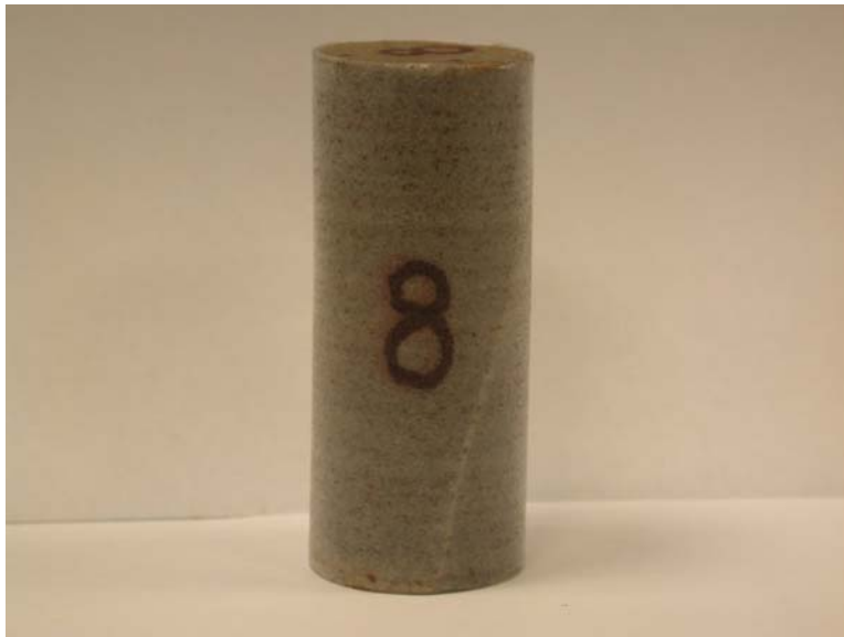
Figure 24: Berea sandstone core after fracturing.
