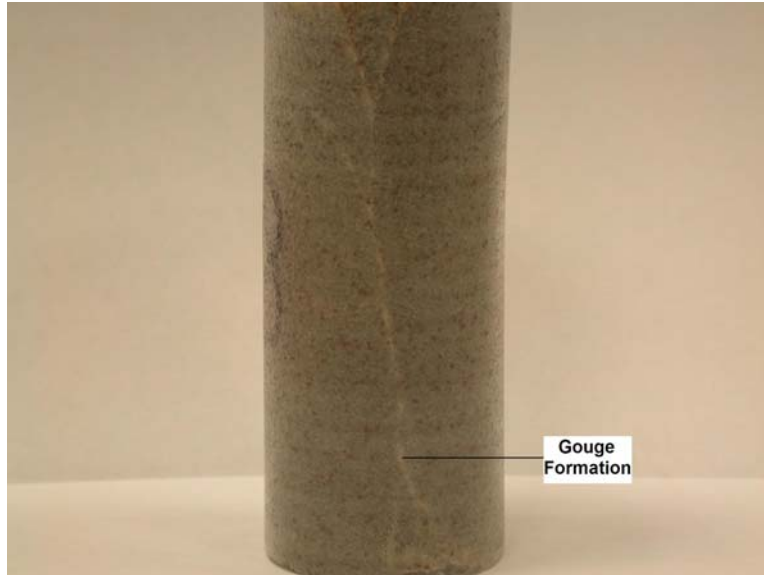
Figure 25: Berea sandstone core after fracturing.
