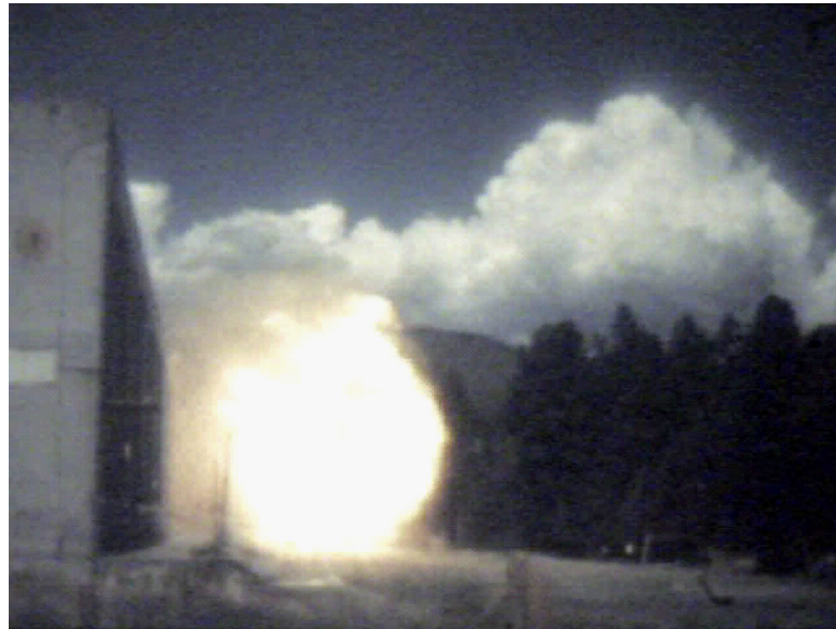
Figure 34: Fireball being pushed out of the bay from a large charge size.
