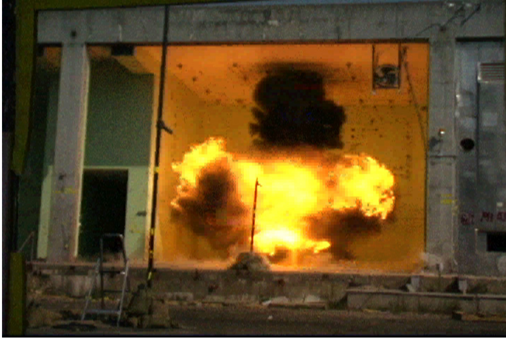
Figure 32: Test video from 5-lb shot showing fireball size.
