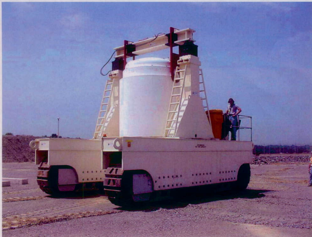
Figure B-6. Site-Specific Cask Transporter
