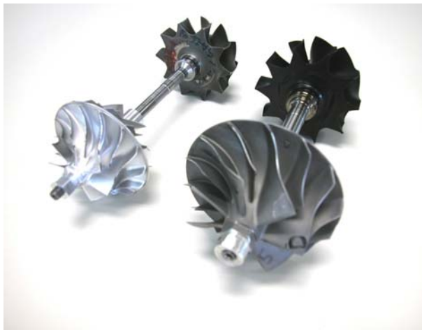
Figure 49: IBT low inertia turbo rotating components compared to conventional turbocharger components of the same flow capabilities
