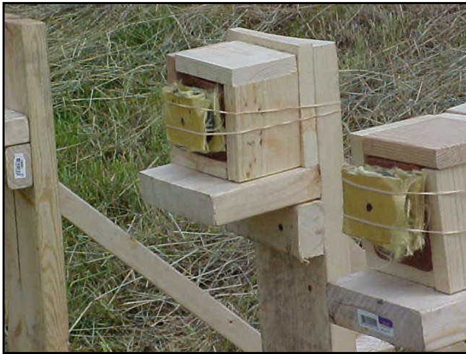
Figure 6. The target setup consisted of a Kevlar/foam sample with a modeling clay backing.
