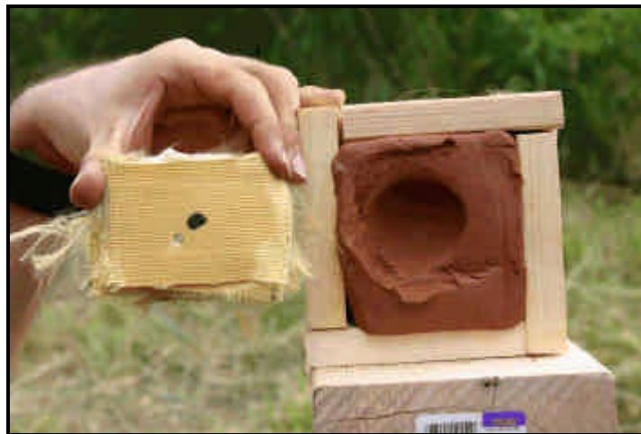
Figure 10. A single ½" thickness of carbon foam backed by Kevlar face sheets was successful at stopping a bullet from a .22 long rifle. The impact crater in the clay was about 0.8" deep and was considered a success.
