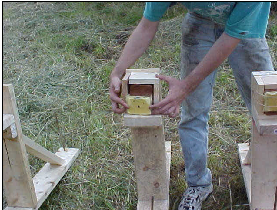
Figure 8. Overview of test setup showing clay behind layered sample.
