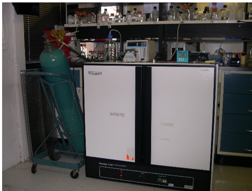
a) External View of Incubator, CO 2 Supply and pH Control System
