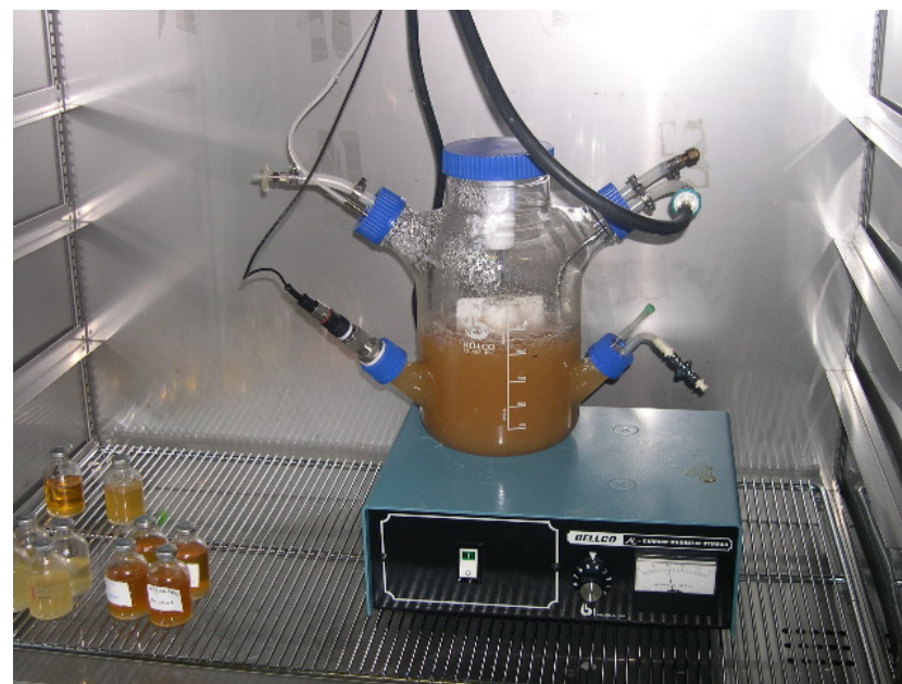
b) Modified 3 L Spin Flask, Stirrer, and Maintenance Cultures
