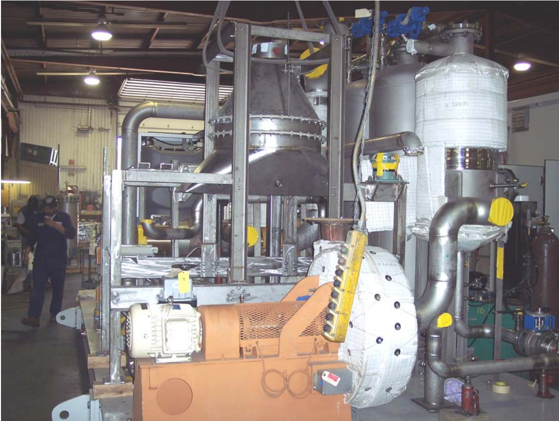
Figure 3. Fuel Treatment Skid Fabrication
