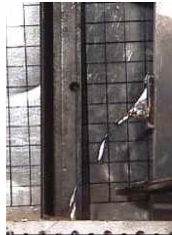
Figure 69: Flow of Aluminum out of a 1.3 mm Web
