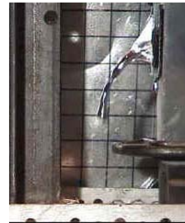
Figure 71: Flow of Aluminum out of a 1.3 mm Web
