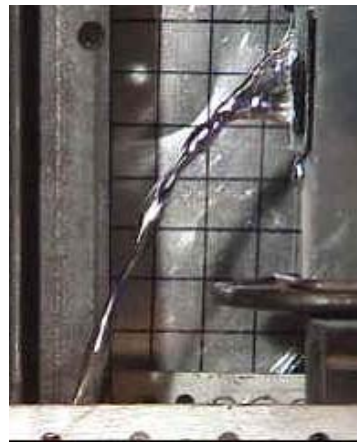
Figure 71: Flow of Aluminum out of a 1.3 mm Web
