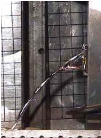
Figure 69: Flow of Aluminum out of a 1.3 mm Web
