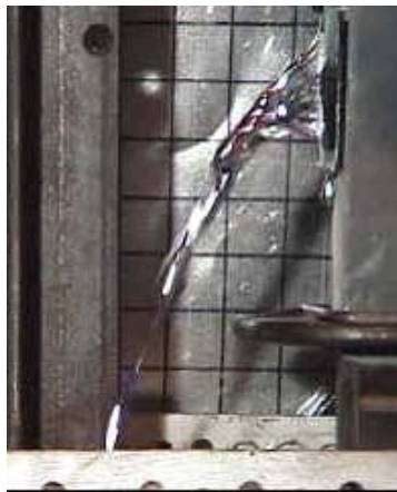
Figure 71: Flow of Aluminum out of a 1.3 mm Web
