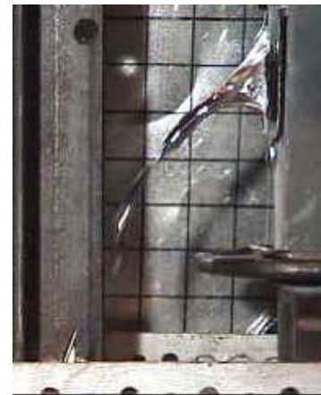
Figure 71: Flow of Aluminum out of a 1.3 mm Web
