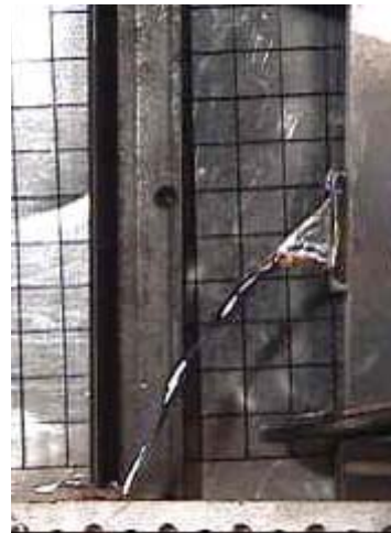
Figure 69: Flow of Aluminum out of a 1.3 mm Web
