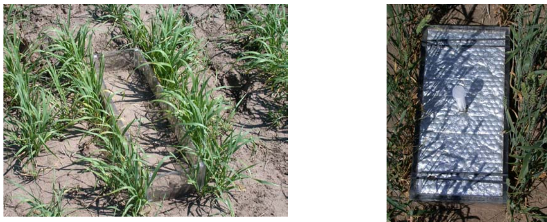
Figure 4. Nitrous oxide gas samples are collected using a vented chamber made of plexiglass. Without cover (left). With cover (right)
