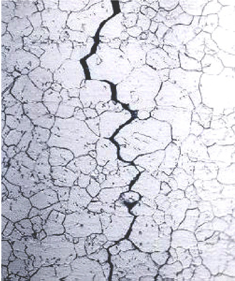
Figure B-2. Typical Example of Intergranular Stress Corrosion Cracking in Stainless Steel
