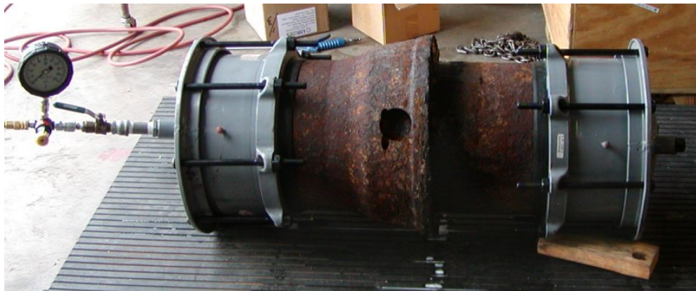
Figure 14. Cast Iron Joint Tested for Leaks
