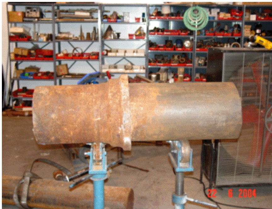
Figure 8. 12-Inch Cast Iron Pipe Sample
