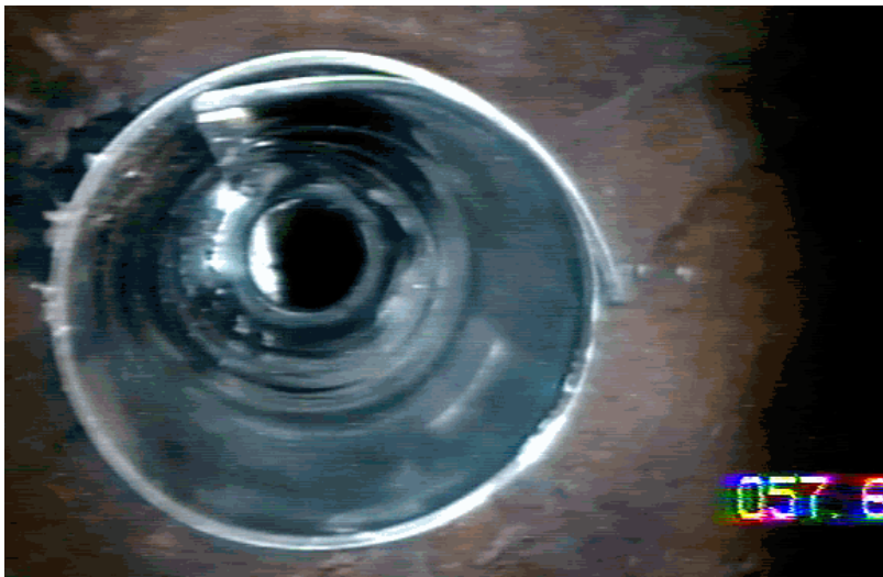
Figure 45. Partially Engaged Patch at 58.6 ft
