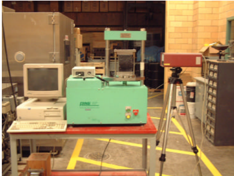
Figure 8-4: Overall setup of indirect tension test
