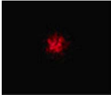
Figure 3-91. Far Field Radiation Pattern from Output of Clad Sapphire Fiber
