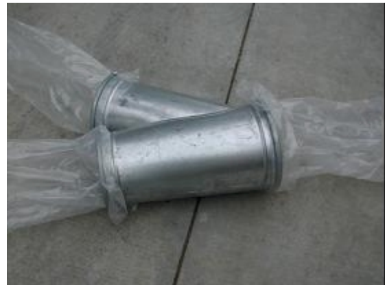
Figure 2.3.1: Wye splits aerosol flow between supply and return
