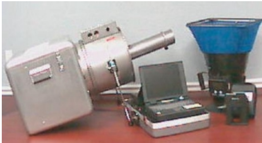
Figure 2.1.1: Aeroseal sealing machine, computer-control suitcase, and diagnostic tools (flow capture hood, and infrared laser-guided temperature-measurement gun)
