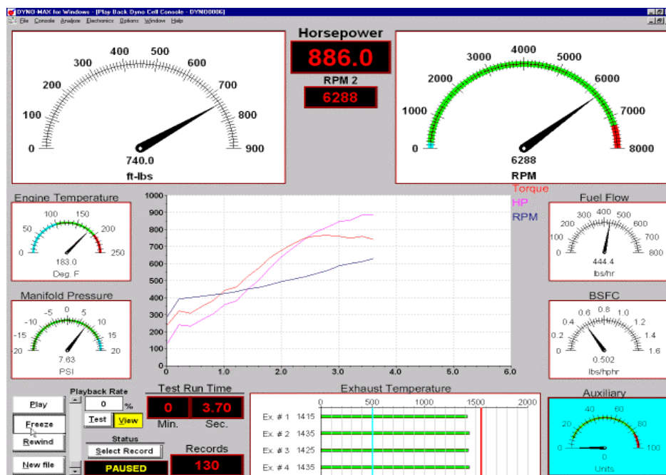
Figure 1. Example of the parameters that are now monitored in the engine test facility.
