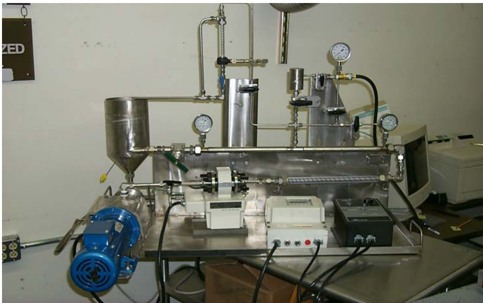
Figure 2. Bench scale cross flow filtration system for accelerated filter membrane erosion.
