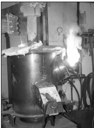
Figure 17: Static Bed VRR Experiment in a Single Electrode Arc Furnace.
