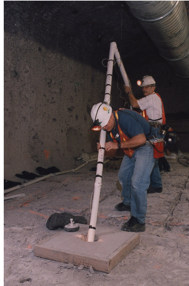
YM-20706 Acoustic Tomography Testing Activities In Alcove 8.
