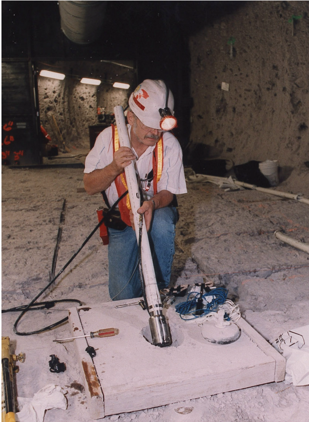
YM-20704 Acoustic Tomography Testing Activities In Alcove 8.
