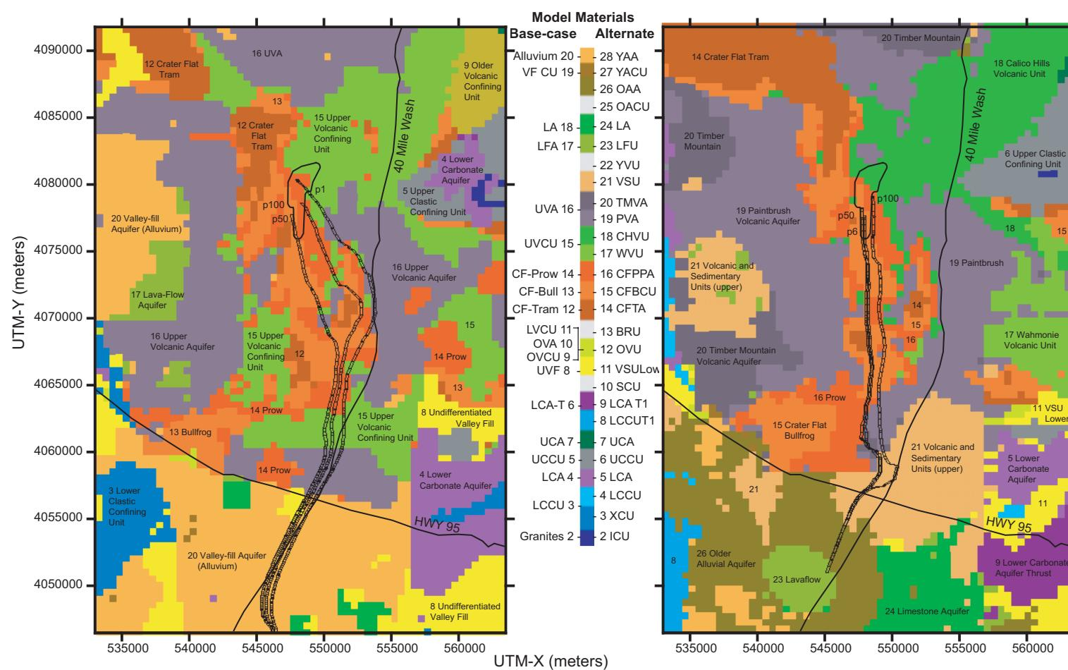
Source: Base-case site-scale SZ flow model grid (HFM-19) DTN: LA0304TM831231.002 [DIRS 163788] (left), Alternate site-scale SZ flow model AM0 grid (HFM-27) DTN: LA0409GZ831231.001 [DIRS 171605].
