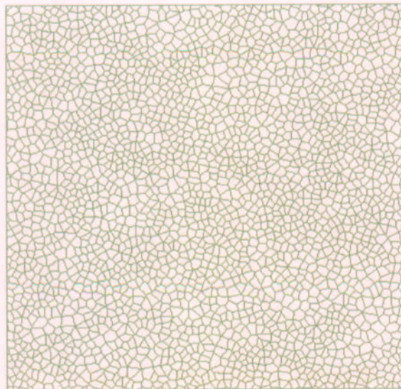
Figure 1 UDEC rock “sample” composed of irregular blocks bonded with frictional and cohesive interfaces
