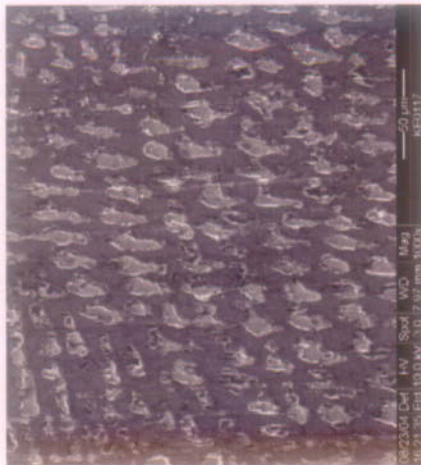
Figure 10: Interdentritic etching in the creviced area of Alloy 22 tested in 0.0005 M NaCl at 90°C. Mag. X 1000.
