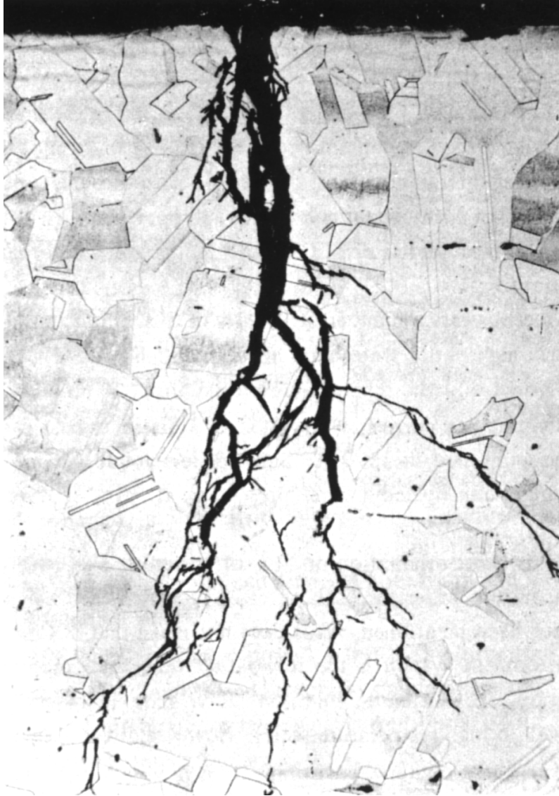
Figure 6.3-2. Typical Example of TGSCC in Stainless Steel
