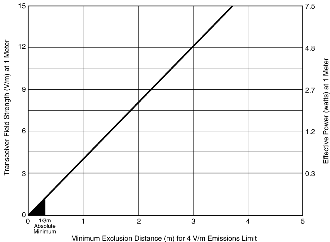
Figure 4-1 Recommended Minimum Exclusion Distance (in Meters) as a Function of Transceiver Field Strength (V/m) at 1 Meter
