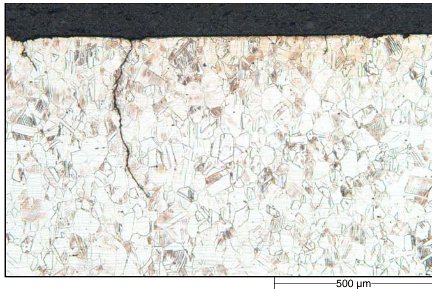
Figure 4-15 Typical view of microstructure with transgranular crack originating from external surface.
