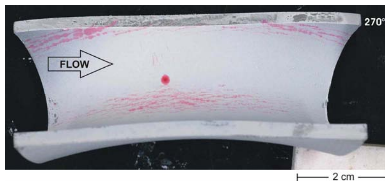
Figure 6-12 Internal surface of intrados showing multiple axial cracking and the defect causing leakage in the form of a spot-like indentation in the middle of the halfshell.
