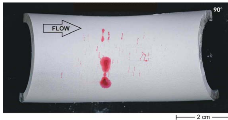
Figure 6-11 External surface of intrados showing array of circumferential cracks.
