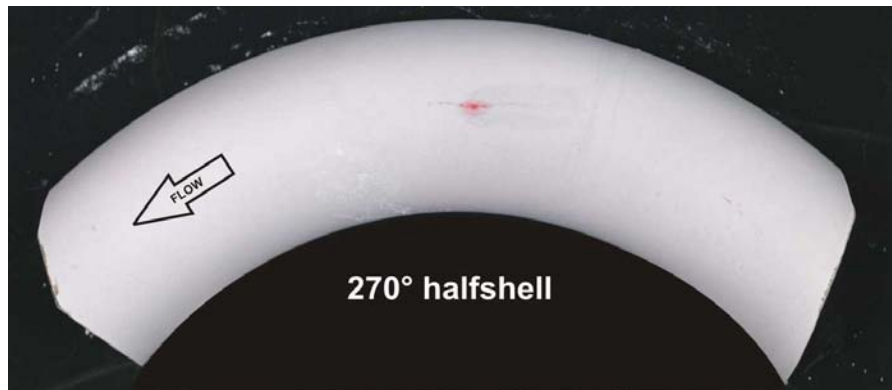
Figure 9-12 External surface at 270° position revealing axial through-wall defect.
