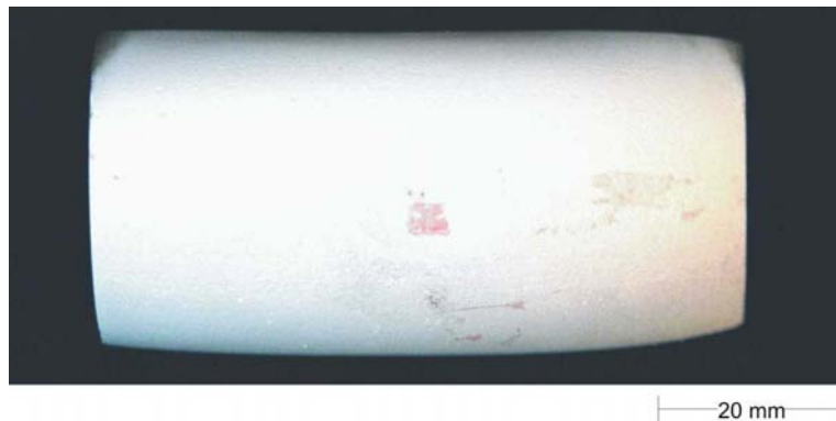
Figure 5-14 No indications found on external surface of the extrados.
