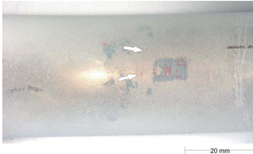
Figure 10-17 External surface of intrados showing fine circumferential cracking as indicated by white arrows.
