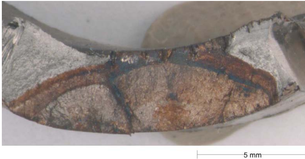
Figure 5-17 Broken open circumferential crack used for fractography.
