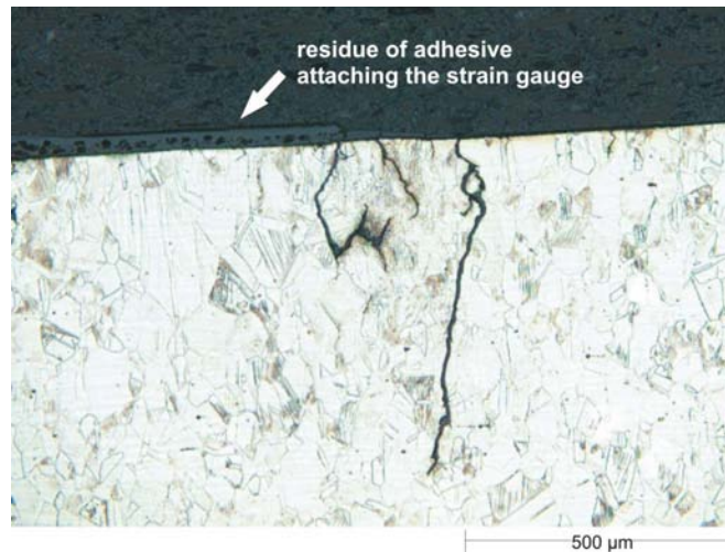
Figure 4-16 Transgranular cracking in area where strain gauge was positioned.
