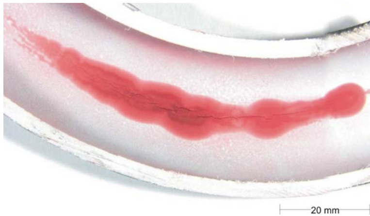
Figure 10-16 Internal 90° position confirming multiple axial cracking (approximate length 60 mm).
