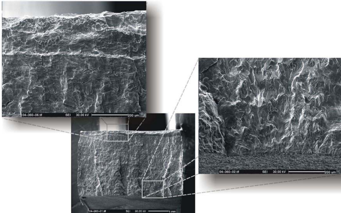
Figure 11-17 Different stages of crack progression confirming corrosion fatigue at 270° position.
