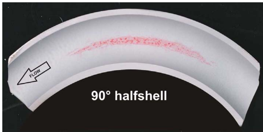
Figure 9-14 Internal surface at 90° position revealing multiple axial cracking.
