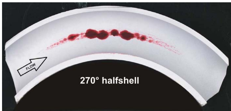
Figure 9-13 Internal surface at 270° position revealing multiple axial cracking.
