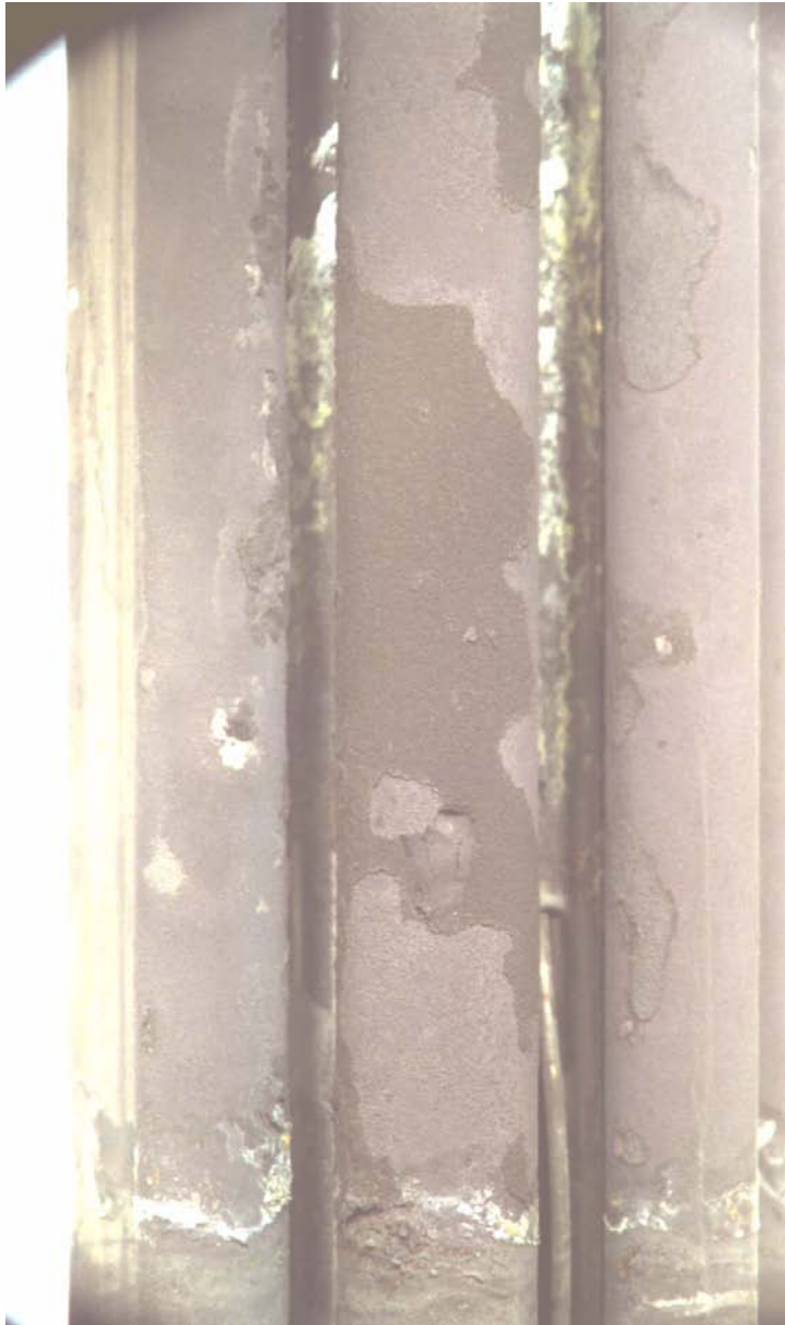
Figure 9-1 Crud deposits on upper section of fuel bundle
