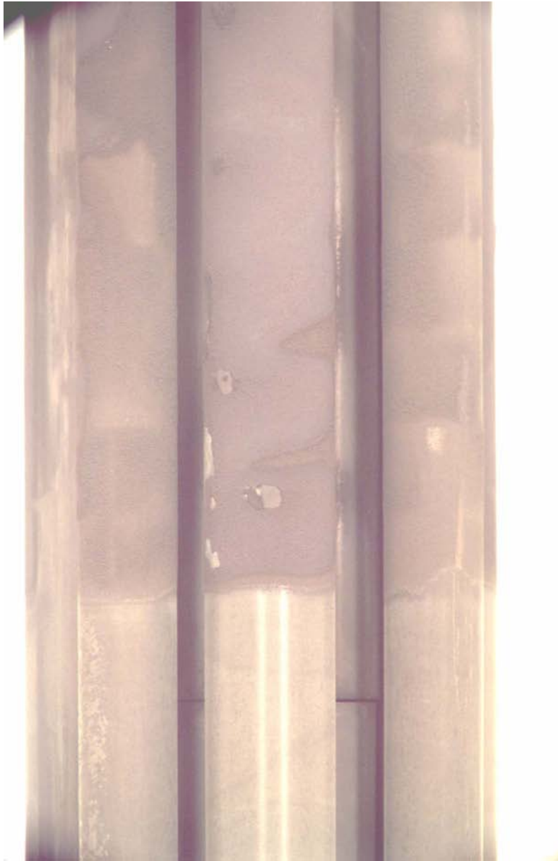
Figure 9-2 Photograph showing crud deposition commencing at boundary between low and high enrichment fuel
