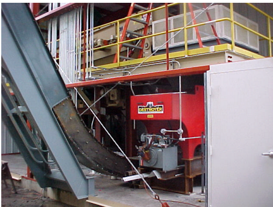
Figure 6-4. The disc screen and overs grinder discharge to the outfeed conveyor
