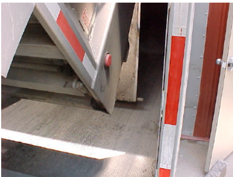
Figure 9-2. The lack of tailgate clearance for coal trucks at the Albright demonstration
