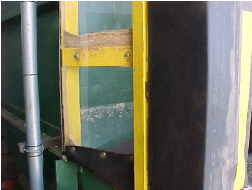
Figure 6-3. The plexiglass and rubber bumper structure at the sawdust receiving hopper, designed to minimize spillage
