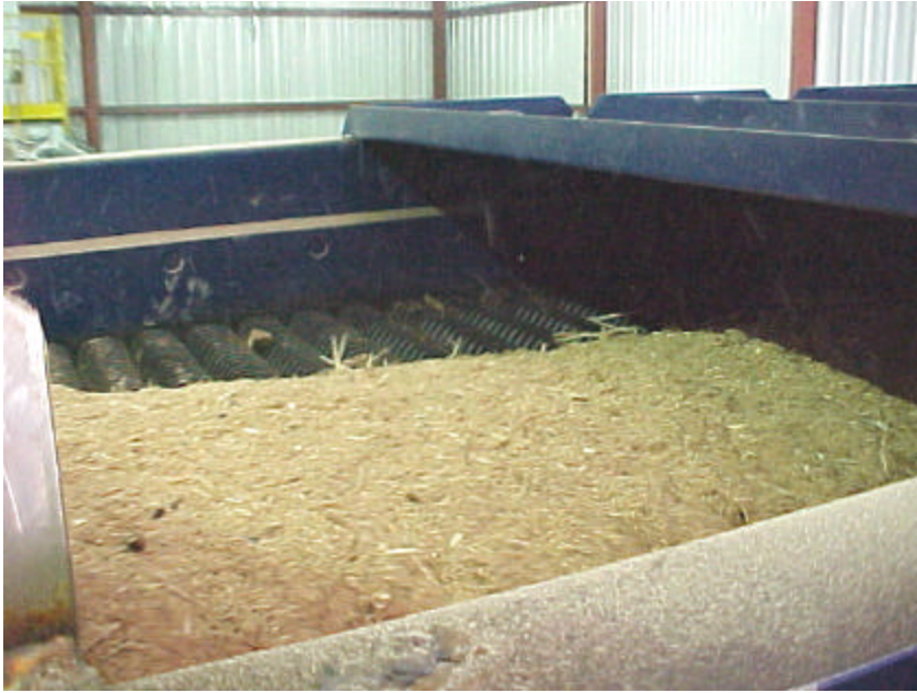
Figure 8-4. Sawdust being screened on the disc screen at Albright
