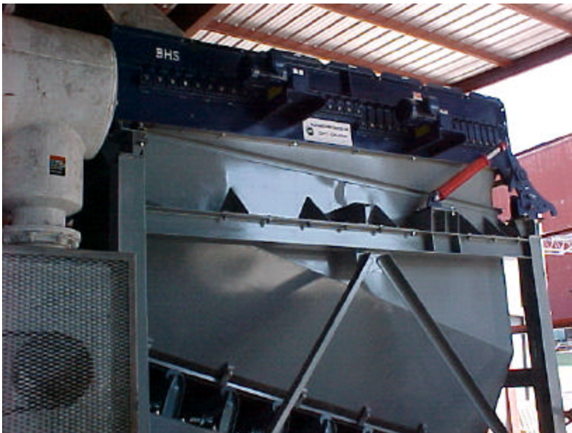
Figure 7-7. The 30 disc screen installed at the Albright demonstration. Note that the building has not been completely enclosed at this point
