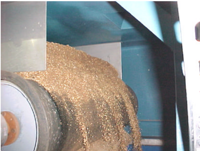
Figure 8-4. Sawdust being screened on the disc screen at Albright
