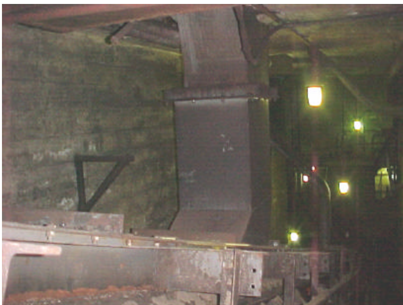
Figure 6-9. The discharge chute feeding sawdust onto the main conveyor at Willow Island Generating Station
