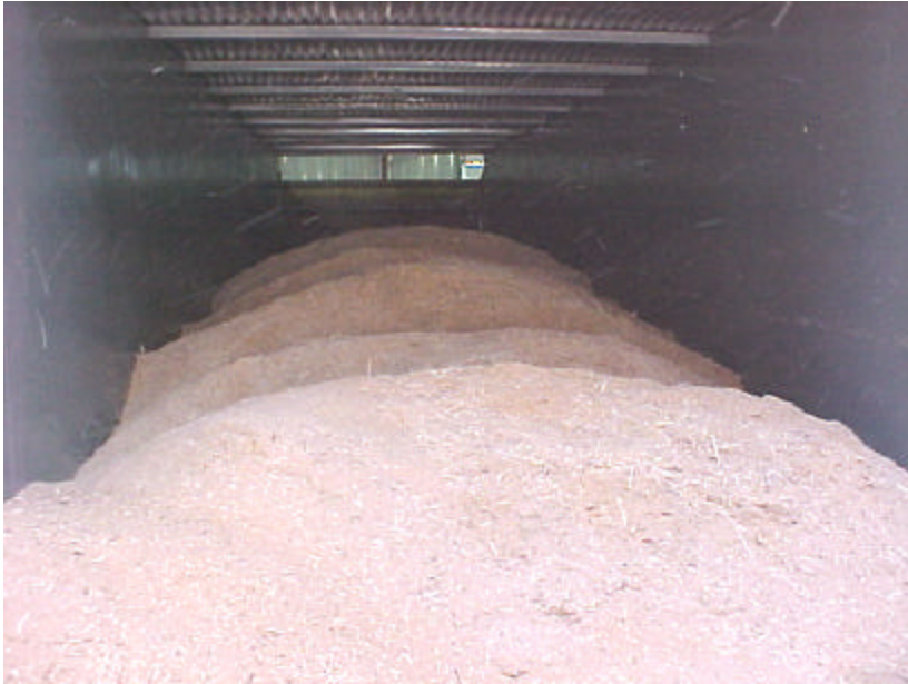
Figure 8-2. Sawdust being transported up the walking floor unloader at Albright
