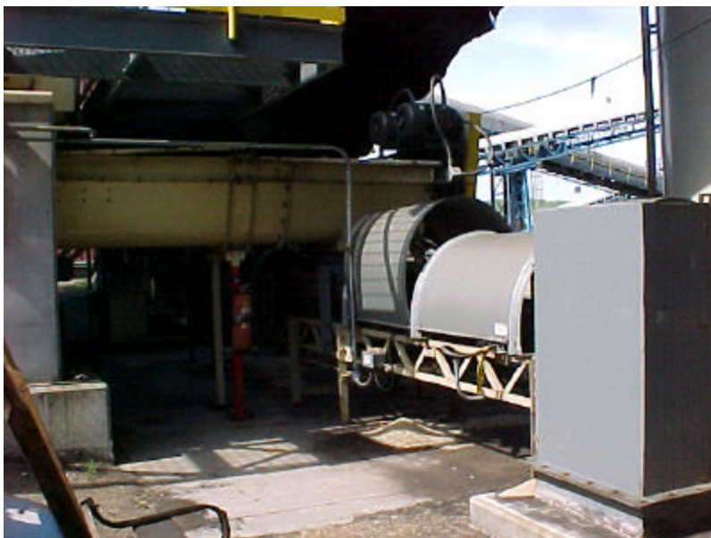
Figure 6-8. The discharge of the twin auger conveyor to the metering weigh belt conveyor at Willow Island Generating Station
