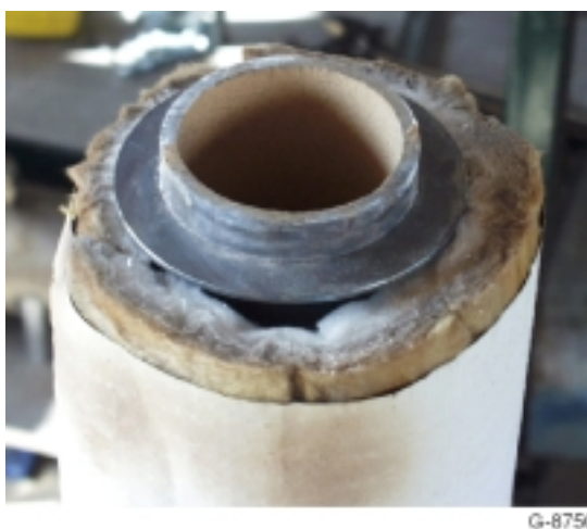
Figure 7. Top end of the new pipe and ashcan assembly. The diameter of the pipe matches the inner diameter of the combustion chamber's retort thus eliminating restrictions at the exit of the combustion chamber.
