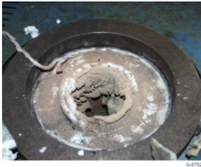
Figure 9. Photograph of the diffuser at the top of the combustion chamber showing accumulation of ash and unburned coal powder.
