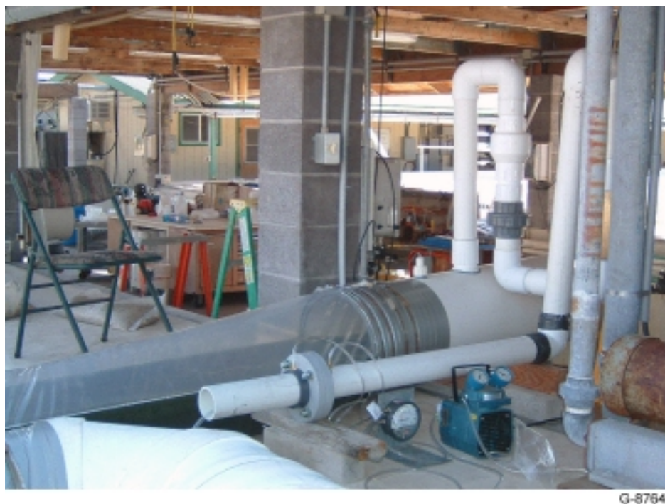
Figure 21. Photograph showing the gas sampling system and the orifice meter attached to the photobioreactor vent at the Mera Pharmaceuticals facility.
