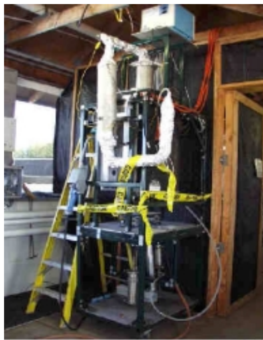
Figure 5. The custom built coal reactor used to provide actual flue gases to the cultures in the photobioreactors.
