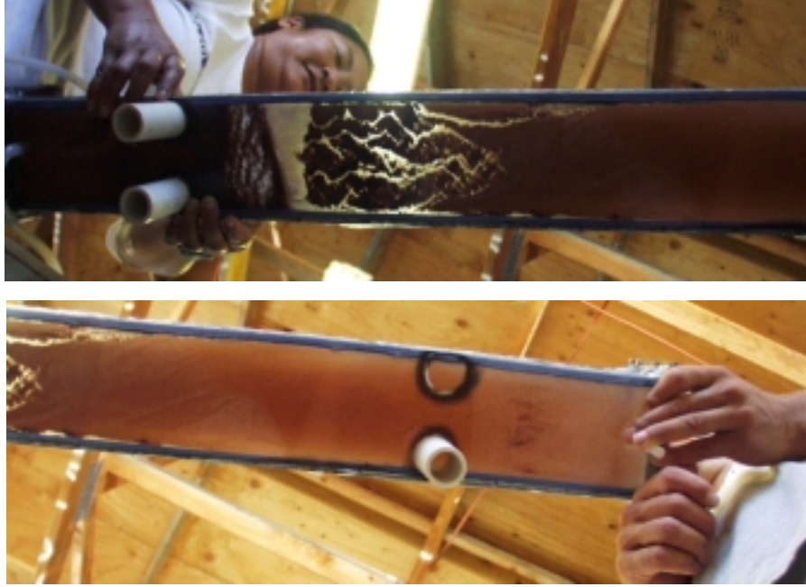
Figure 18. Photographs of the bottom of the unit after draining showing the pattern of settled cysts near the inlet (top) and outlet (bottom) ports.
