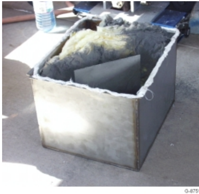
Figure 8. Inside view of the new ashcan. Its larger capacity permits us to carry out longer duration coal burns.
