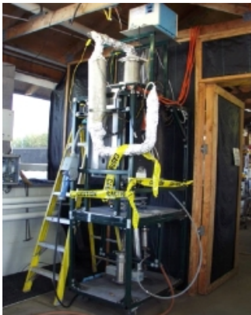
Figure 2. Custom built coal reactor used to generate flue gases used in microalgal carbon capture experiments.
