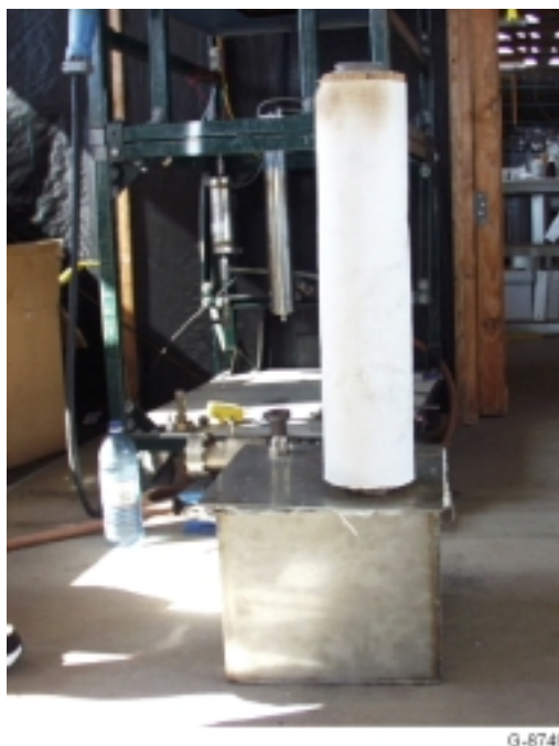
Figure 6. Photograph of the new exit pipe and ashcan assembly constructed for the coal combustor. The larger diameter of the pipe has allowed us to eliminate the recurring blockage from the reactor's exit with slag and ash.
