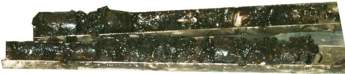
Fig. 3 – Sidewall core samples (ten 1-inch diameter samples) collected September 29, 2004, from 3 Lower Wilcox coal beds penetrated in a well drilled by Anadarko Petroleum Corporation.
