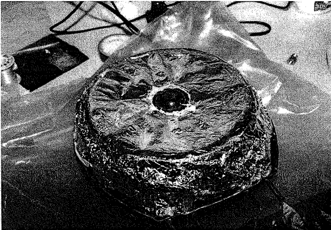
Figure 5.2-35: Multi Layer Insulation Applied to Inner Vessel
