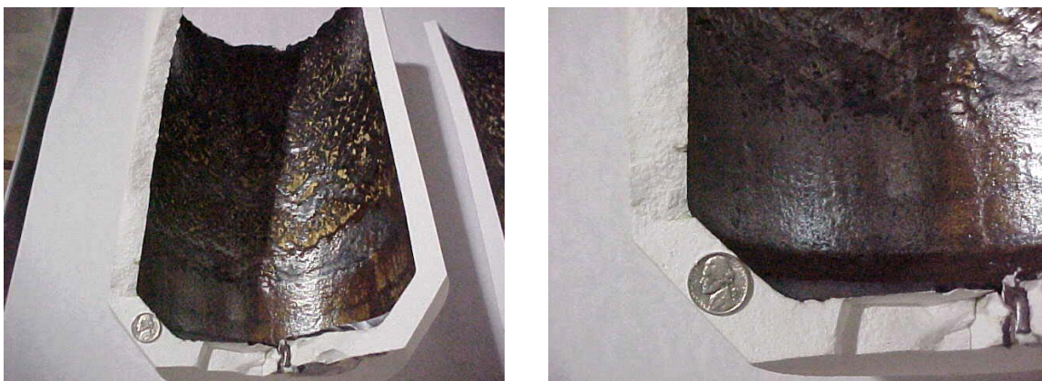
Figure 3. Cross sectional view of a dense high silica crucible (DFC 83% silica 17% alumina) after 14 days at 1250°C with an iron phosphate melt containing 27 wt% Hanford LAW simulant. No significant corrosion was evident on the crucible (Photo courtesy of MO-SCI Corp., Rolla, MO).
