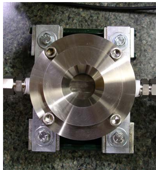
Fig. 11.27 Windowed cell designed & constructed for the ACTF Bubble Characterization Cart
