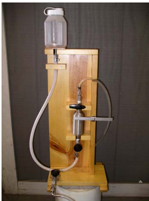
Fig. 11.9 Apparatus for measuring foam quality under system pressure
