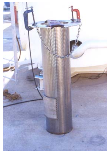
Fig. 3.33 Johnson Screen placed in the separation tower
