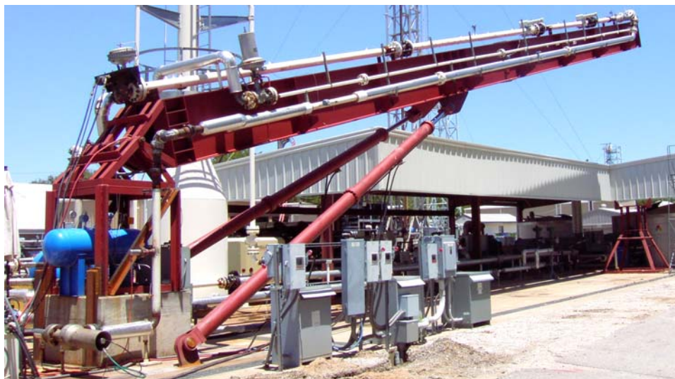
Fig. 3.57 Hydraulic cylinders at approximately 25 to 30 degrees inclination (side view)
