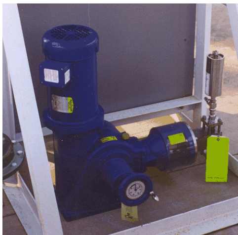
Fig. 3.24 Surfactant injection pump
