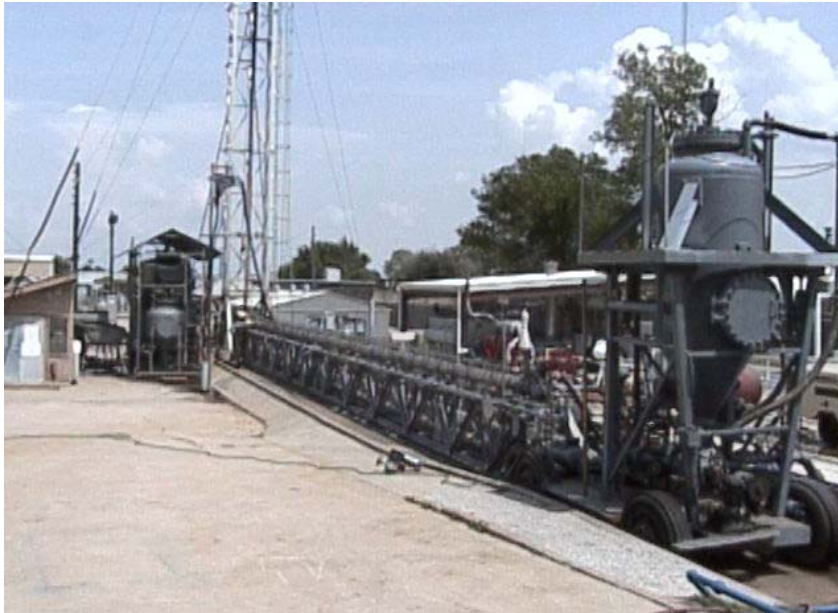
Fig. 4.6 Low pressure ambient temperature flow loop (TUDRP)
