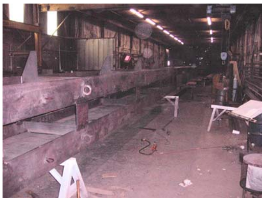
Fig. 3.47 Fabricated new mast
