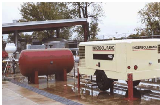
Fig. 3.21 Air compressor and air accumulator tank
