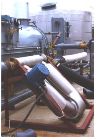
Fig. 3.12 Flow meter ( Micro Motion)
