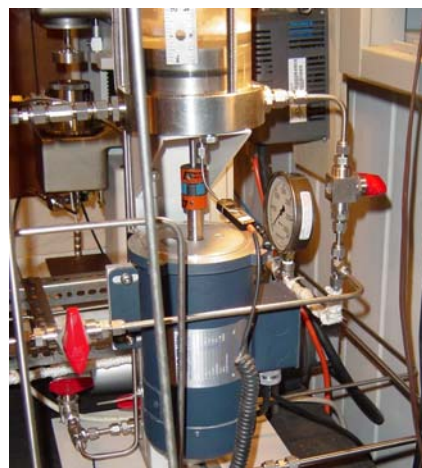
Fig. 8.6 Mixer with variable speed drive
