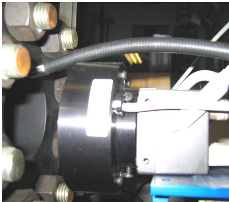
Fig. 11.53 CCD camera with fiber light and ring light installed
