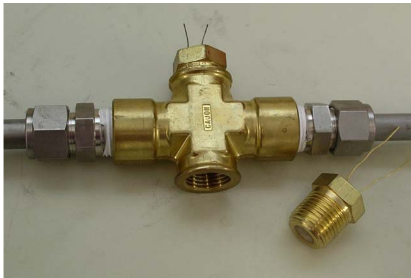
Fig. 11.31 Average bubble size device for use with the Foam Generator-Viscometer
