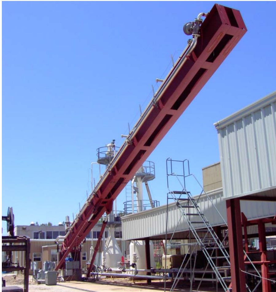
Fig. 3.58 Hydraulic cylinders at approximately 25 to 30 degrees inclination (front view)
