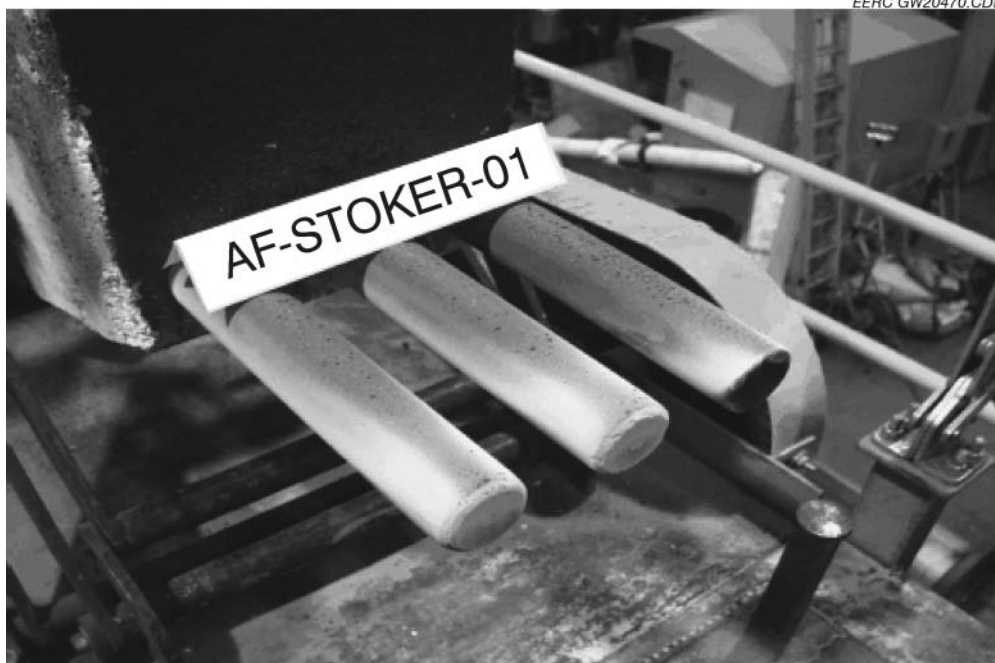
Figure 21. Photograph of fouling probe bank – AF-CTS-Stoker01 – baseline Cordero Rojo.
