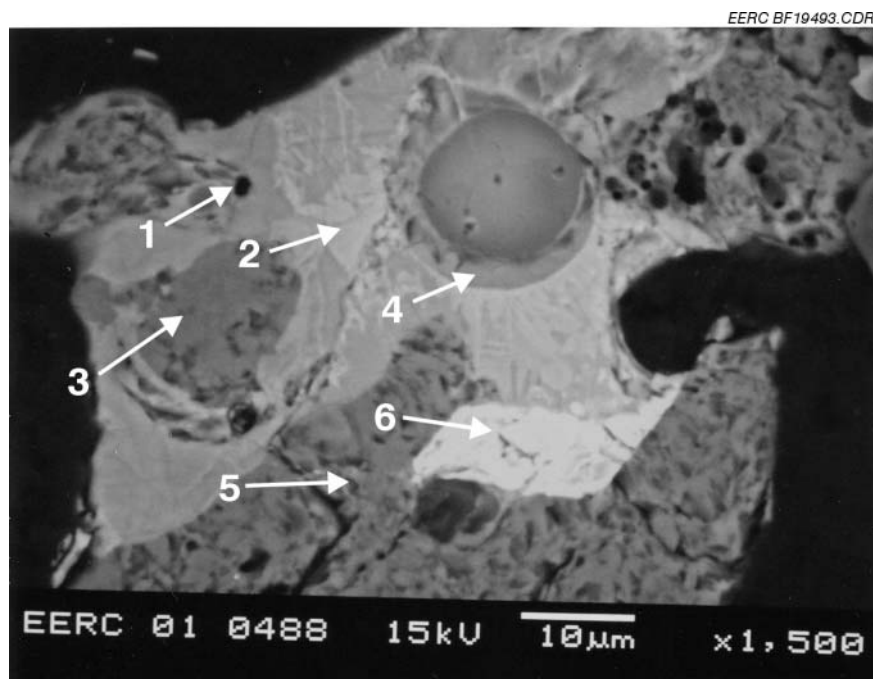
Figure ES-4. SEM micrograph of 80-20 Cordero Rojo-wood chip deposit ash.
