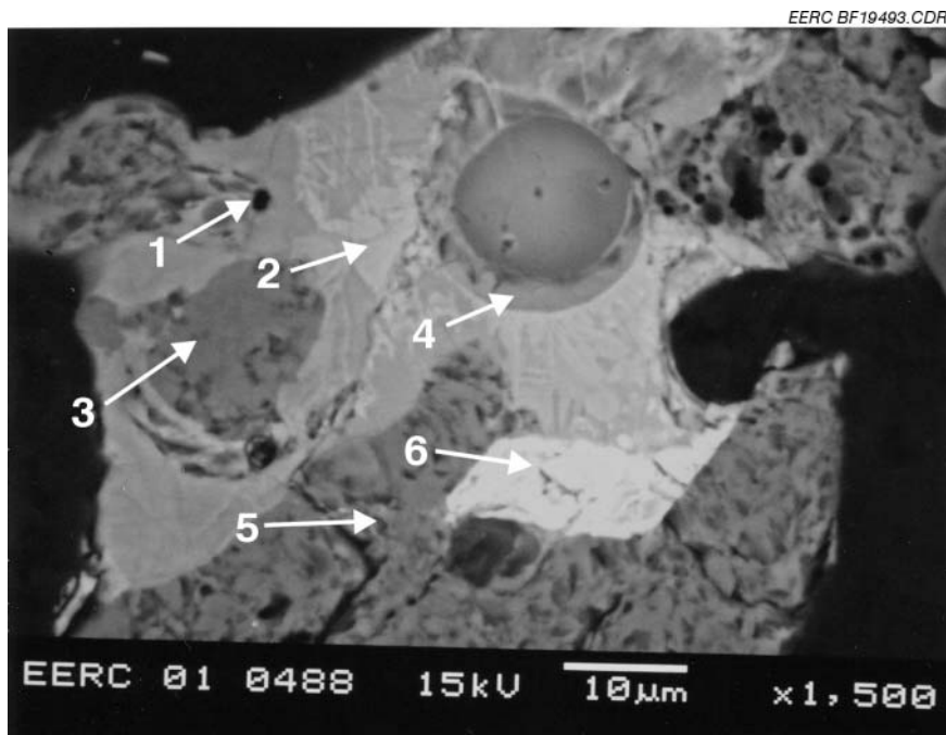
Figure 16d. SEM micrograph of 80-20 Cordero Rojo-wood chip deposit ash.
