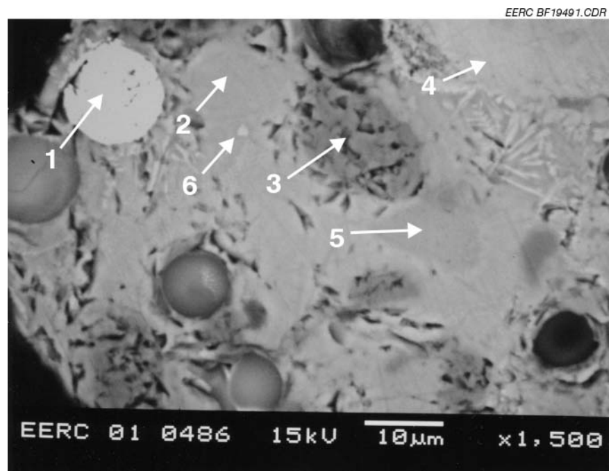
Figure 16b. SEM micrograph of 80-20 Cordero Rojo-sunflower hull deposit ash.
