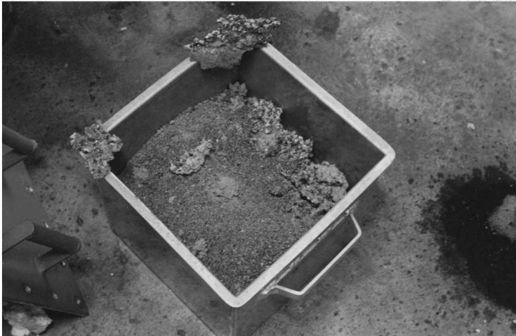
Figure 13. Bottom ash recovered after subsequent grate-fired test.
