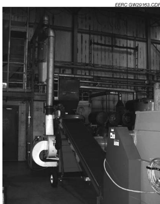
Figure 7. Photographs of hammer mill, blower assembly, and product recovery cyclone.
