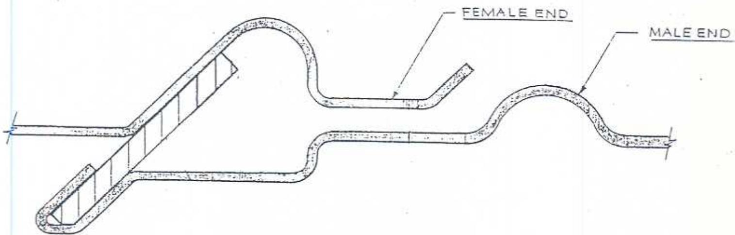
PEG constructed two connection prototypes, a rigid sheet metal duct and a helix core flex duct, and conducted laboratory tests to determine each one's leakage. The first design tested was a 6 inch diameter round sheet metal duct constructed with 26 gauge material. This is the same material used in current residential systems. The second was a helix core flex duct fitting over a 6 inch diameter sleeve.
