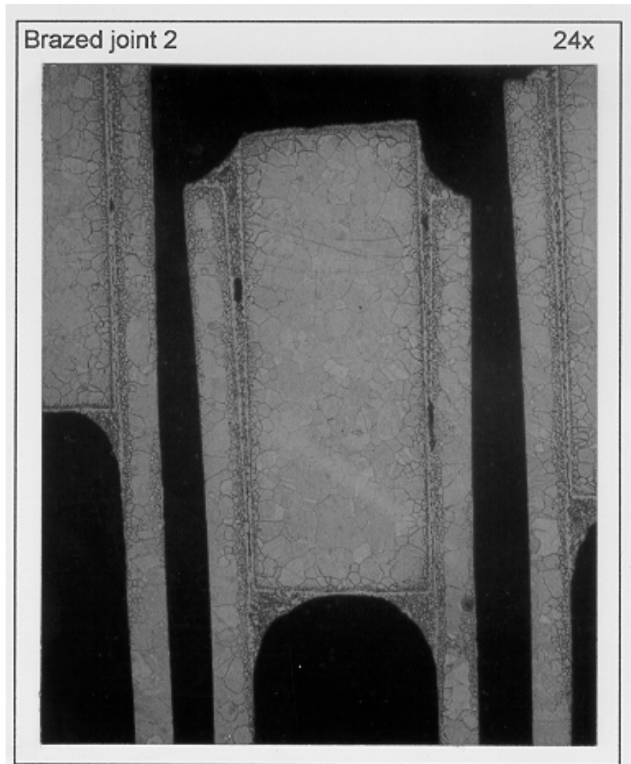
Figure 4.3.2.4.2-4: Good Braze Joint Formation & Reduced Dissolution
