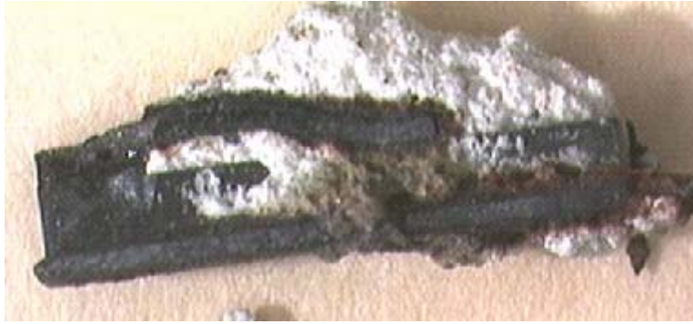
Figure 3.4.3.6-2: X Tip/Connector/Wire Junction Failure
