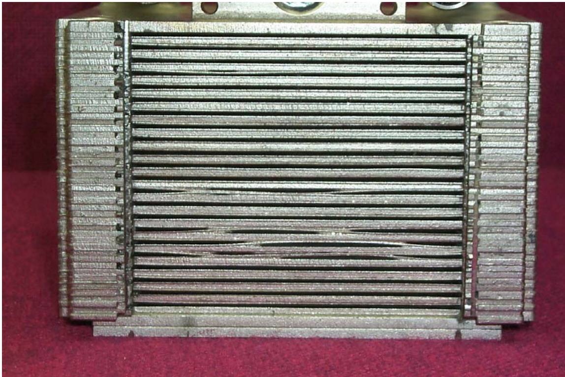
Figure 4.3.2.4.2-6: Front Face of H2 Planar Reformer Showing Separation
