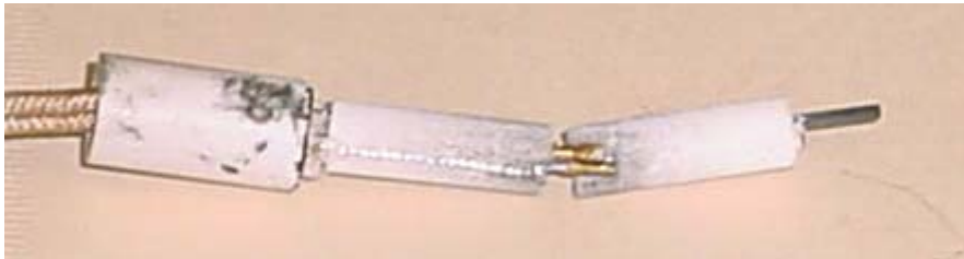
Figure 3.4.3.6-1: Failed Igniter Showing Connection Weakening, Burn Diffusion Along Interface With Tube Shell
