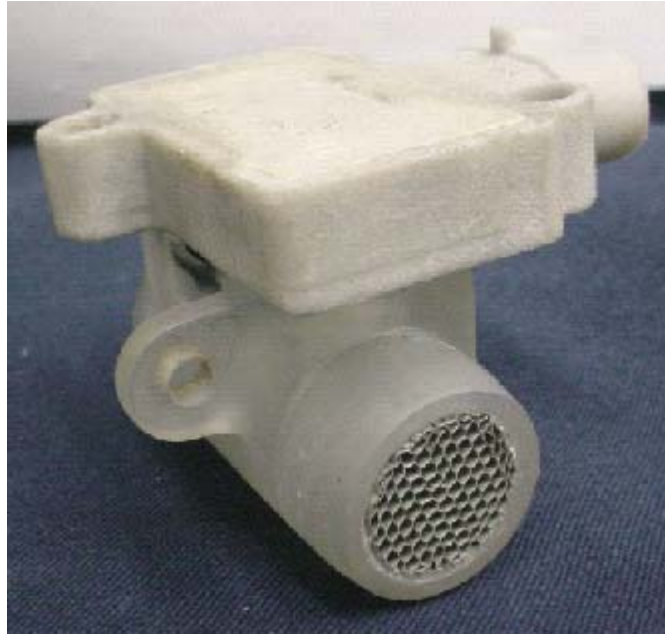
Figure 3.4.2.1-1: Mass Air Flow Sensor Geometry Made From SLA Parts and Integral Honey-Cell Flow Straightener
