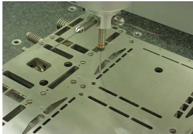
Figure 3.4.3.2-6: ICM Typical Surface Profile Scan
