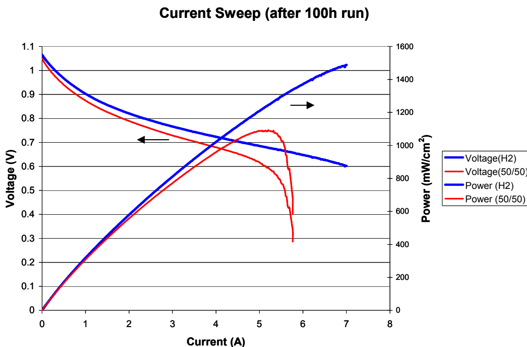
Figure 4.2.4-1: Current Sweep Behavior of LSFCu 2 Under Pure Hydrogen and 50:50 Mixture
