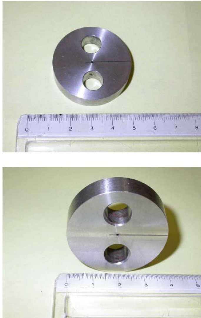
Figure 28. Single edge notch disc specimen
