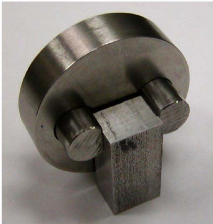
Figure 93. SCC specimen removed from the supercritical reactor.
