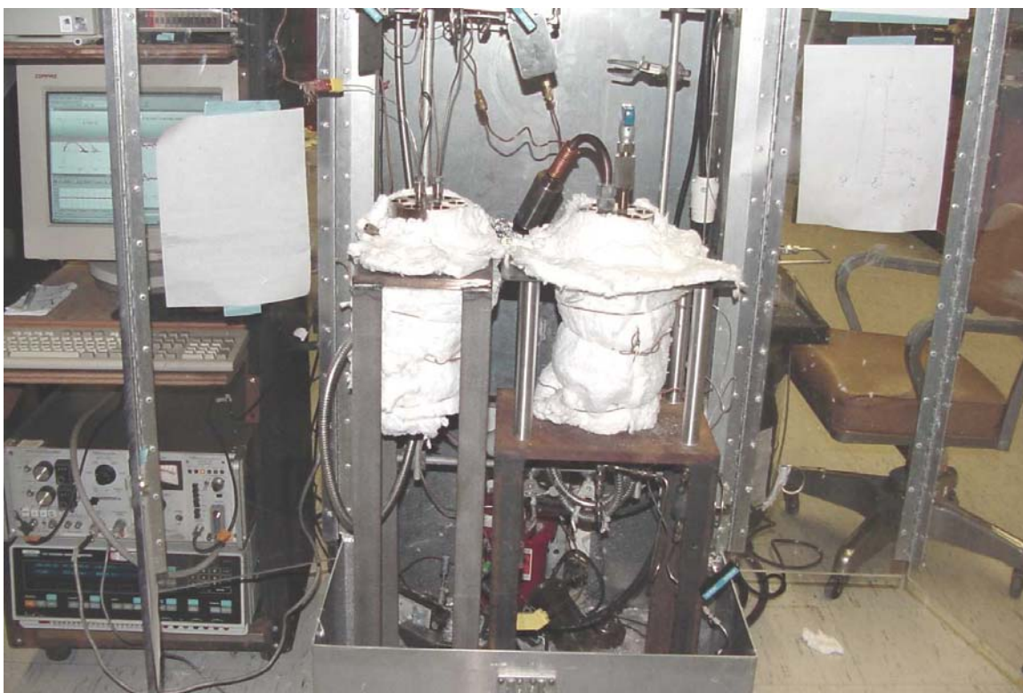
Figure 37. Close view of the APSS reactor (left) and CDE reactor (right)
