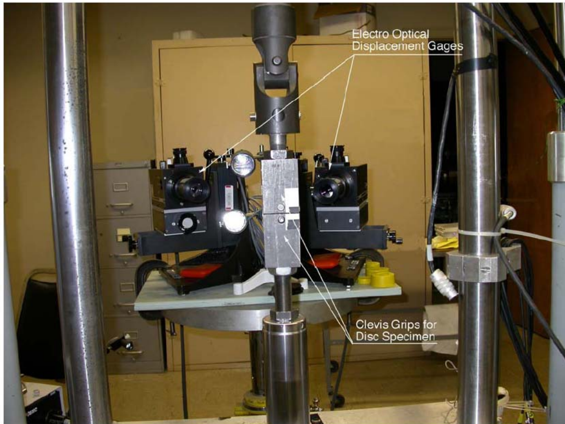
Figure 32. Experimental setup showing two electro-optical displacement transducers.
