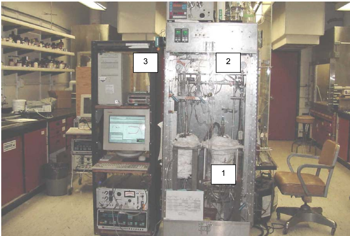
Figure 35. General view of the experimental system: supercritical test reactors (1), the high-pressure loop (2), and the data acquisition system (3).
