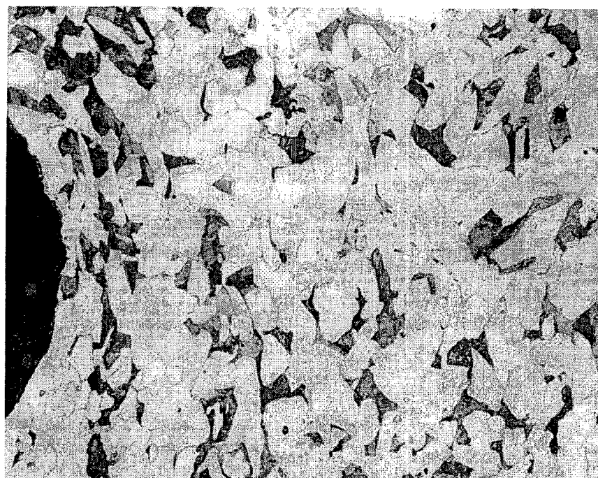
Figure E-12: Test Specimen P-7 – Stress Relieved Microstructure
