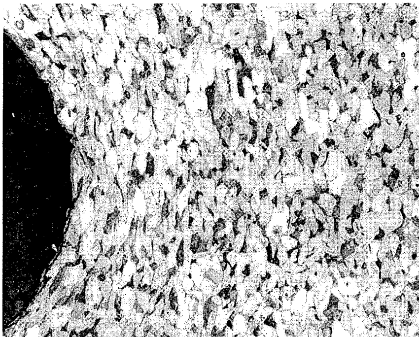
Figure E-4: Test Specimen M-7 – Stress Relieved Microstructure
