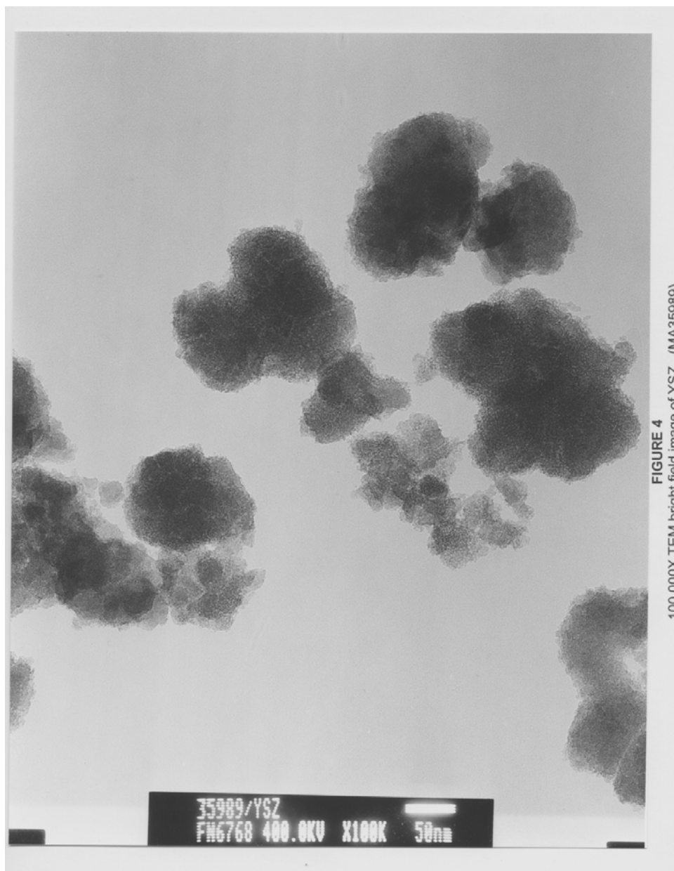
Figure 9: A bright field TEM image of the nanosize YSZ formed by the MD process. The crystallite size is ~5 nm. The agglomerate size in this TEM image is about 50 to 200 nm. The agglomerates are soft, and can be broken with relative ease, down to a few tens of nm.
