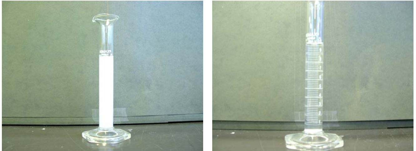
Figure 16: (a) YSZ powder made by the MD process in suspension in water in a measuring cylinder. (b) After the powder had settled down. In Phase I, as much as 100 g of powder was made in a single experiment at each time, using simple lab-ware.
