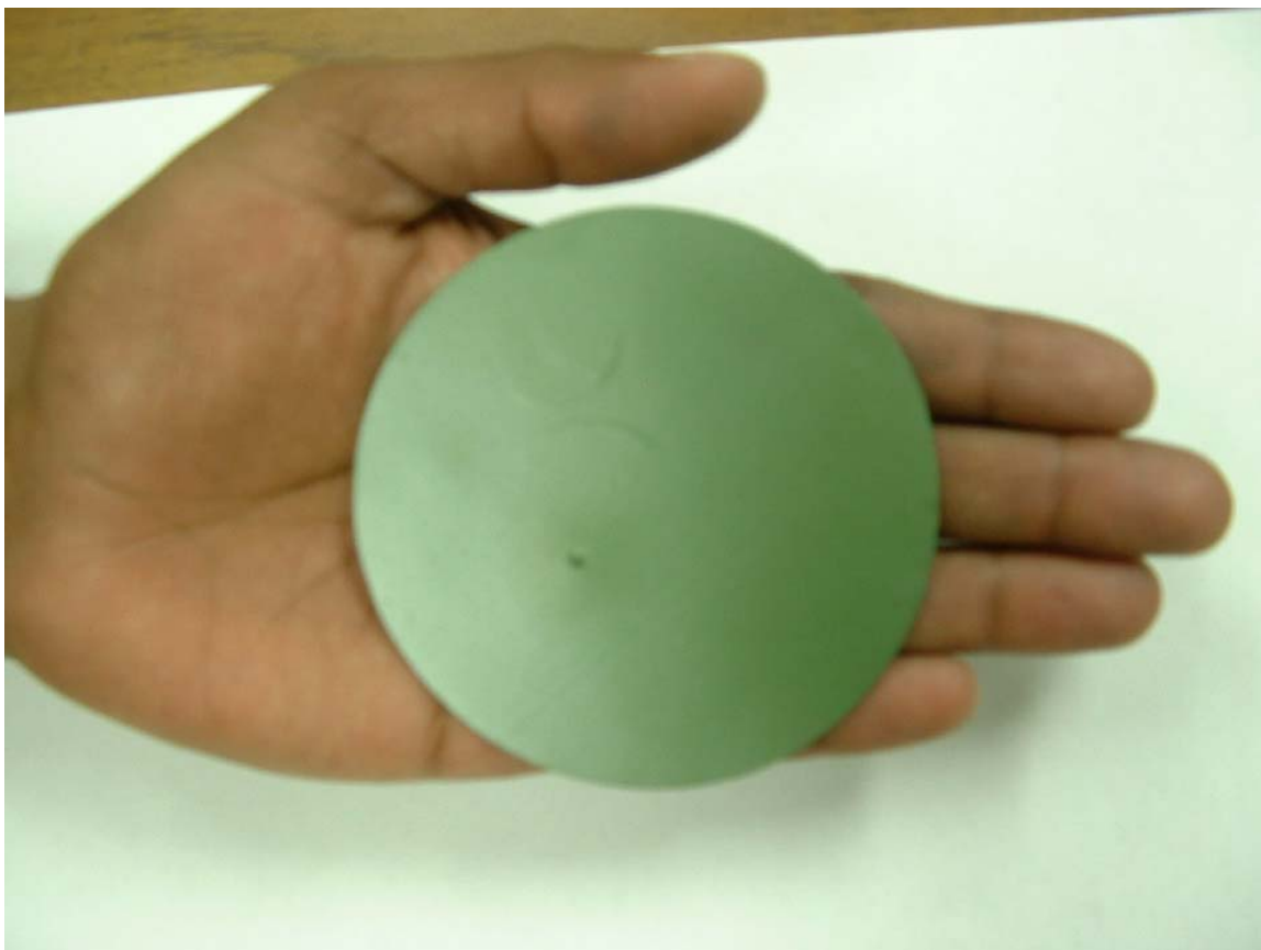
Figure 19: A photograph of an anode-supported cell made with MD-CSZ in the anode support. The cell is over 3 inches in diameter. This cell was made by, die pressing and sintering. In the future, a tape-casting process will be developed.
