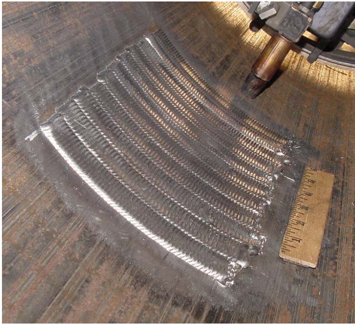
Figure 48 - Finished First Layer of Deposited Weld Metal on Inside Pipe Diameter
