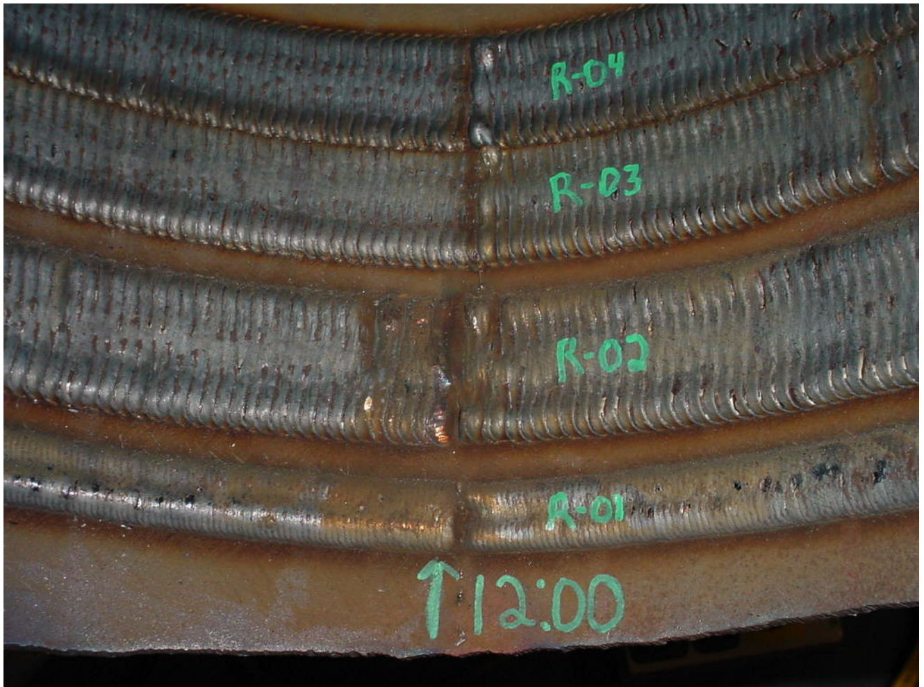
Figure 81 - Tests R-01 through R-04 at 12:00 (Note the Poor Tie-Ins for R-01 through R-03)
