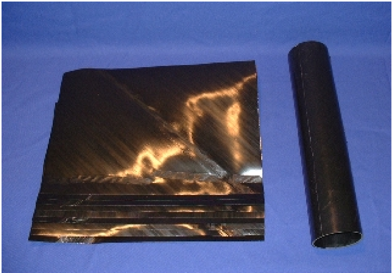
Figure 7 - Lay-Up and Forming of Fiber-Reinforced Composite Liner
