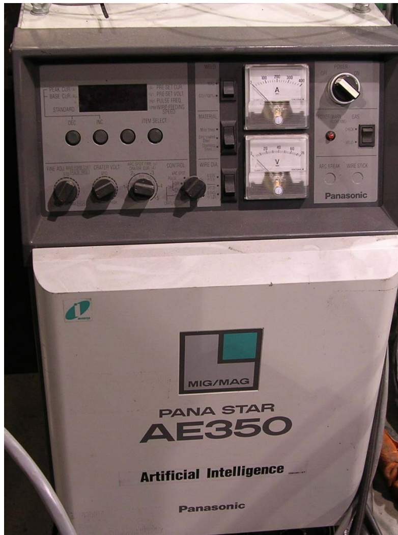
Figure 37 - Panasonic AE 350 Power Supply with Pulse Short-Circuit Metal Transfer Control
