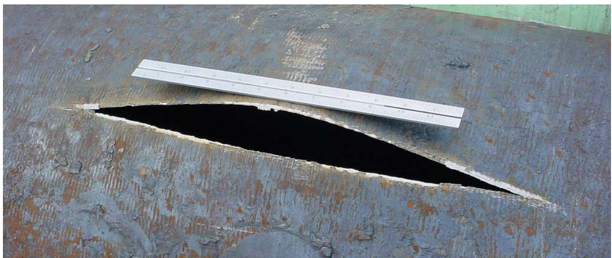
Figure 115 - Hydrostatic Burst Specimen of 558.8 mm (22 in.) Pipe in Virgin Pipe
