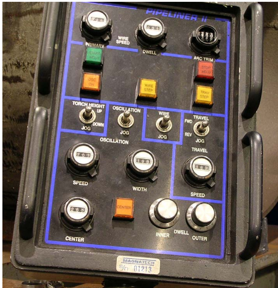
Figure 36 - Magnatech Control Pendant Showing Control Parameters
