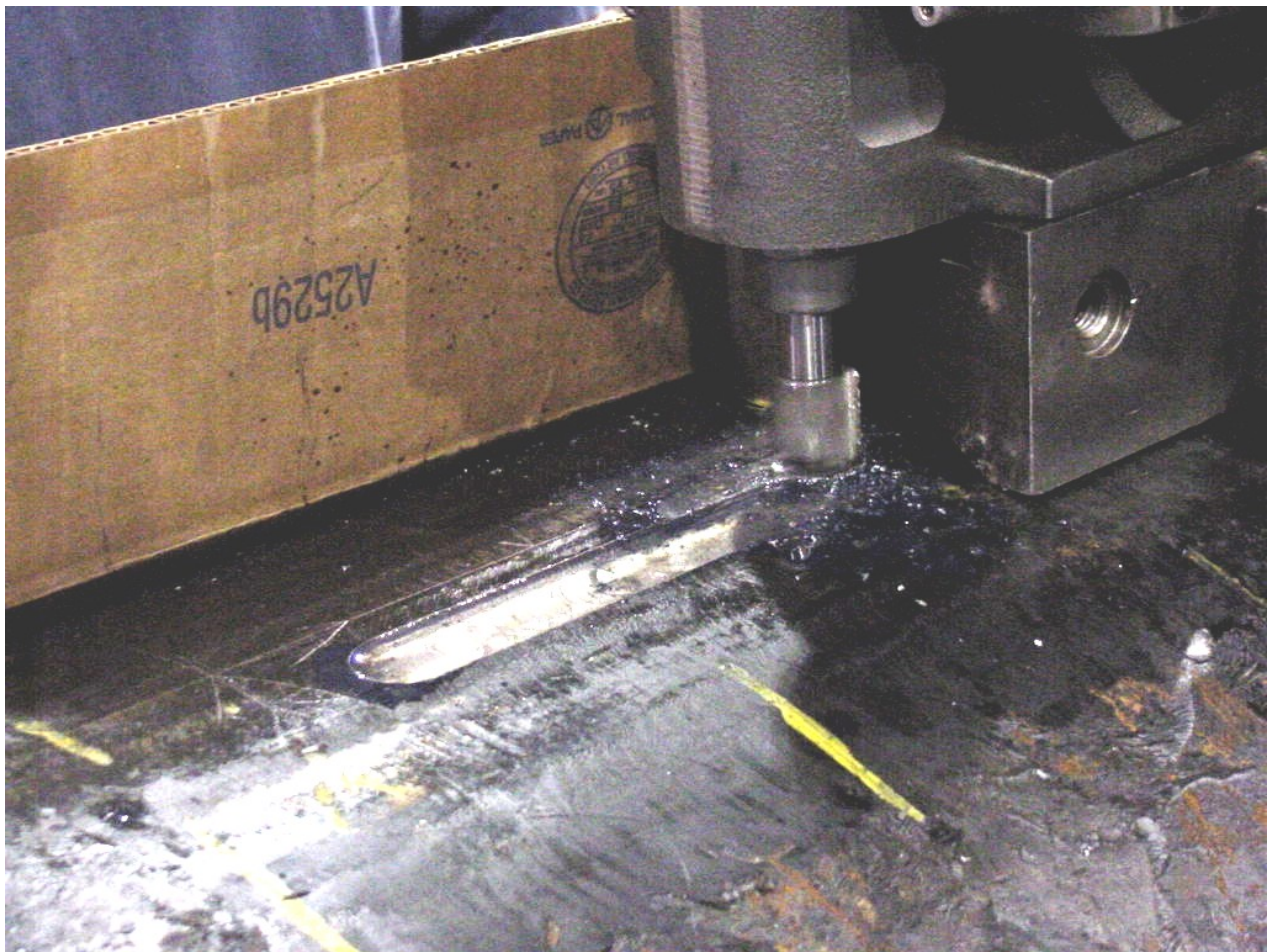
Figure 38 - Milling Machine Set-Up Used to Simulate Corrosion on Pipe Sections
