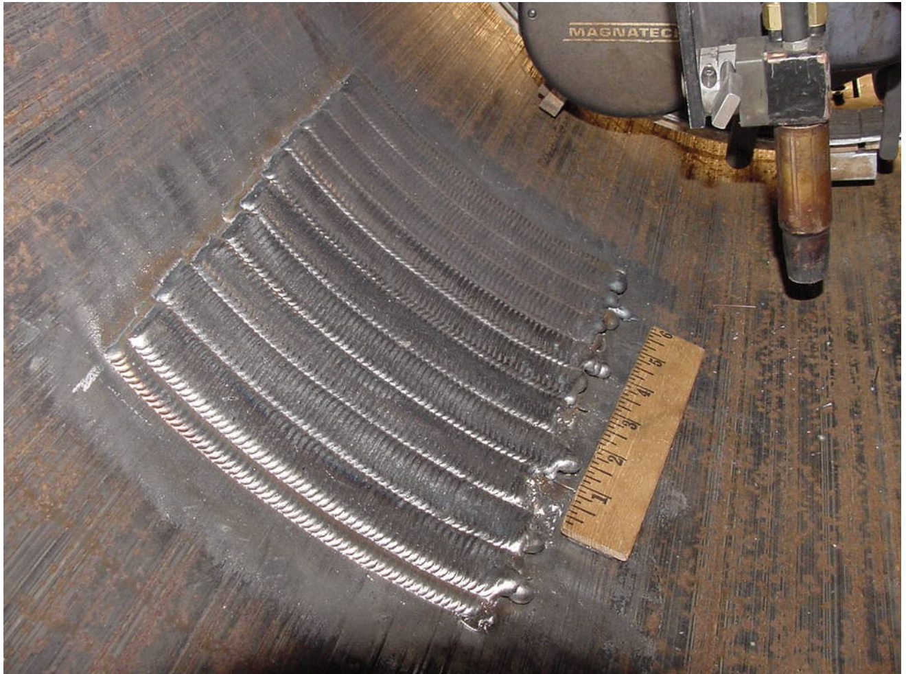
Figure 50 - Finished Second Layer of Deposited Weld Metal on Inside Pipe Diameter
