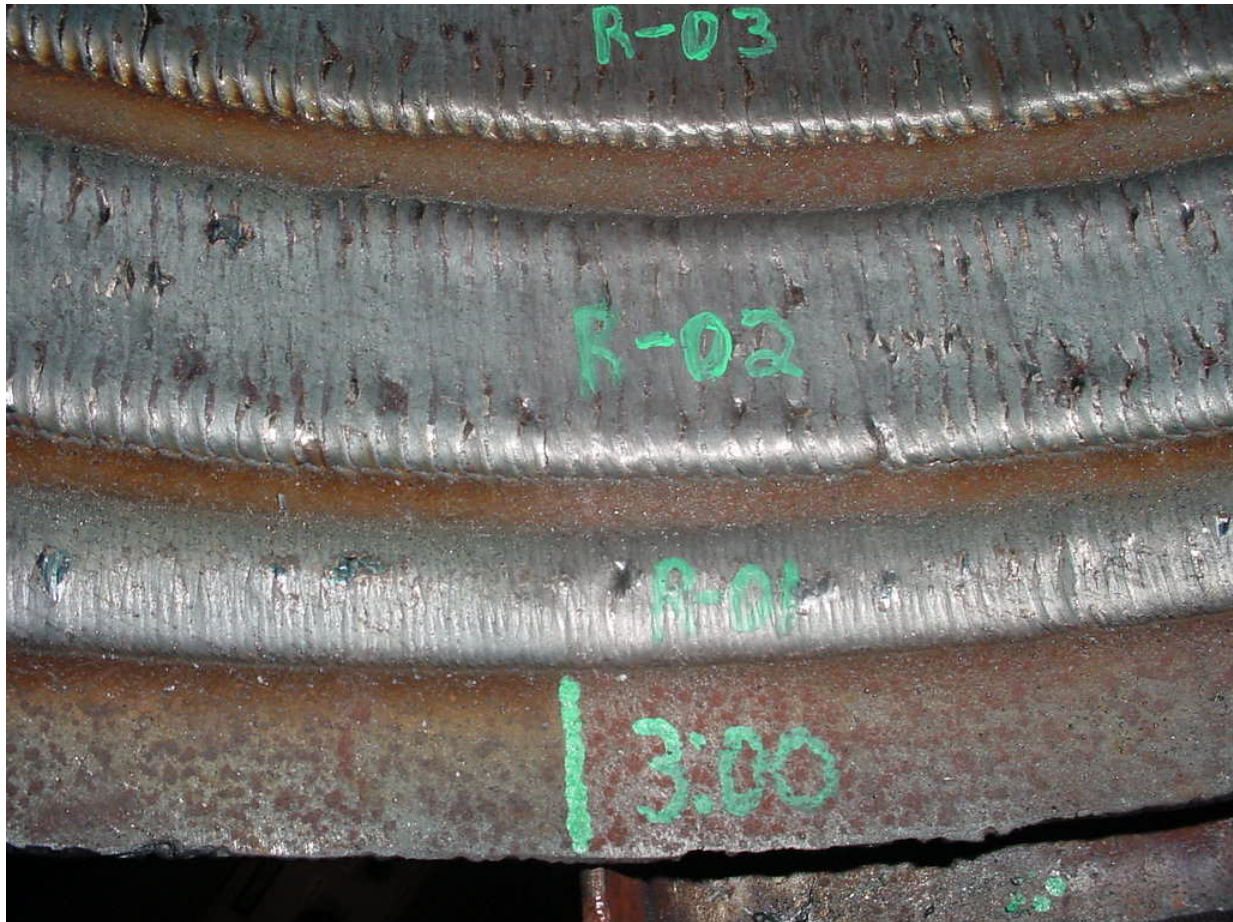
Figure 84 - Tests R-01 and R-02 at 3:00 Showing Steady-State Bead Shape
