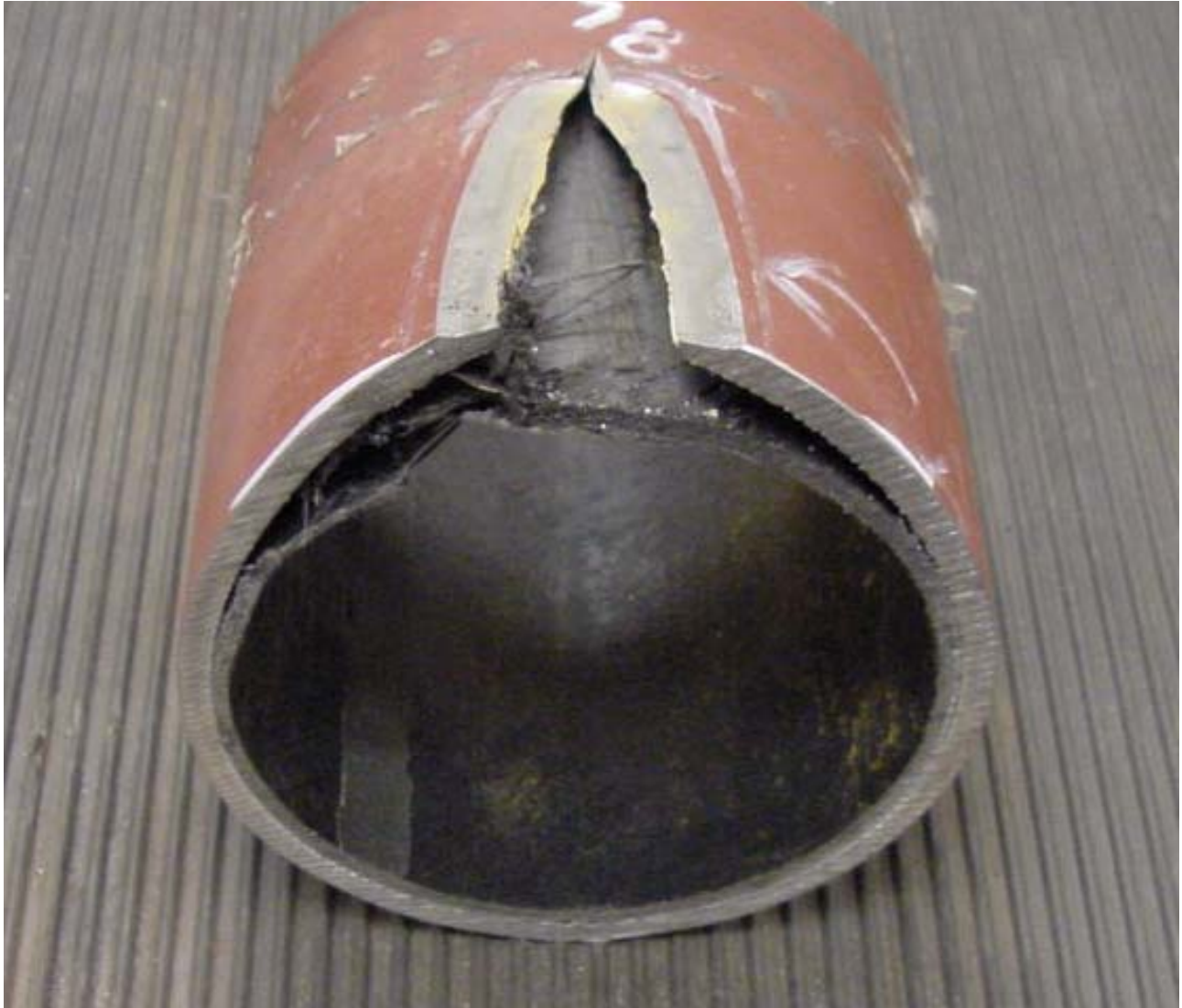
Figure 77 - Water-Jet Cut Section through Pipe Sample Containing Round-Bottom Longitudinal Slot with Liner Installed
