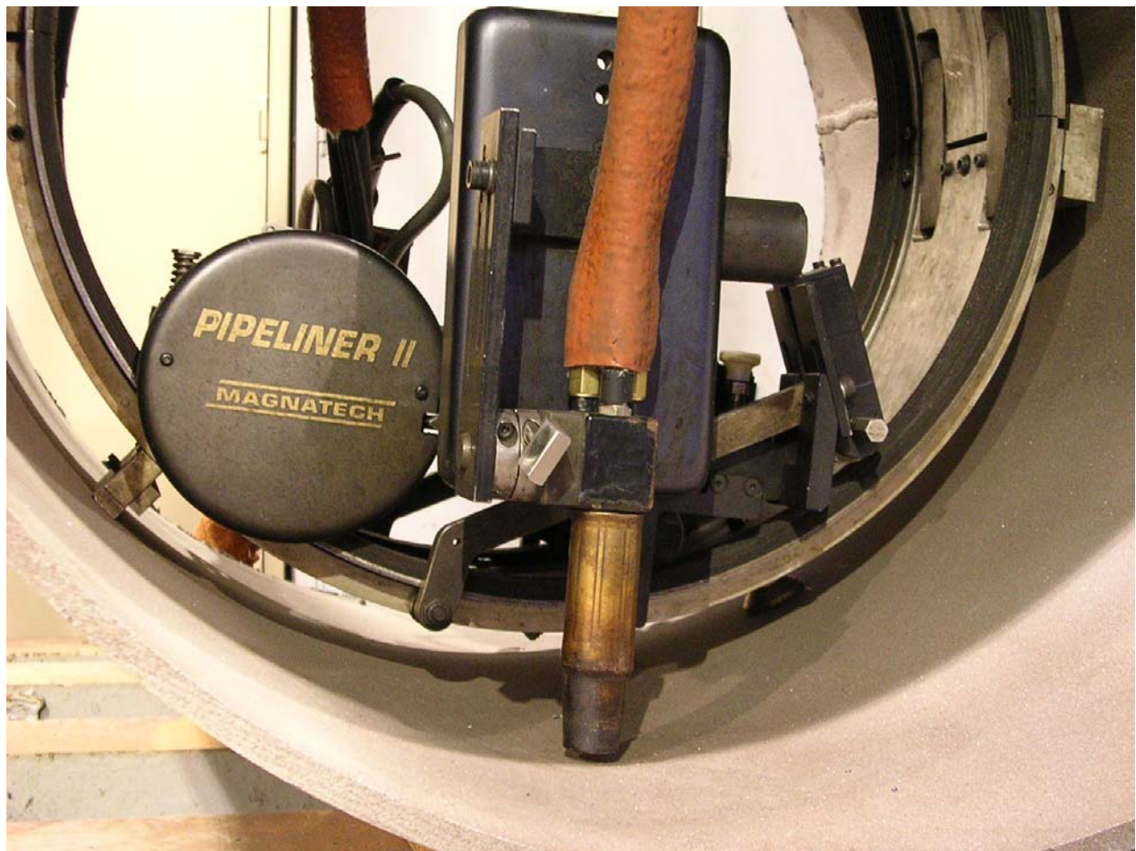
Figure 35 - Magnatech ID Welding Tractor Capable of Spiral & Ring Motion with Oscillation
