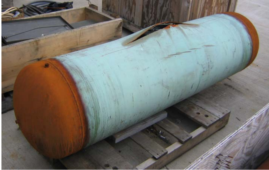
Figure 90 - Pipe With Carbon Fiber-Reinforced Liner Repair After Burst Test
