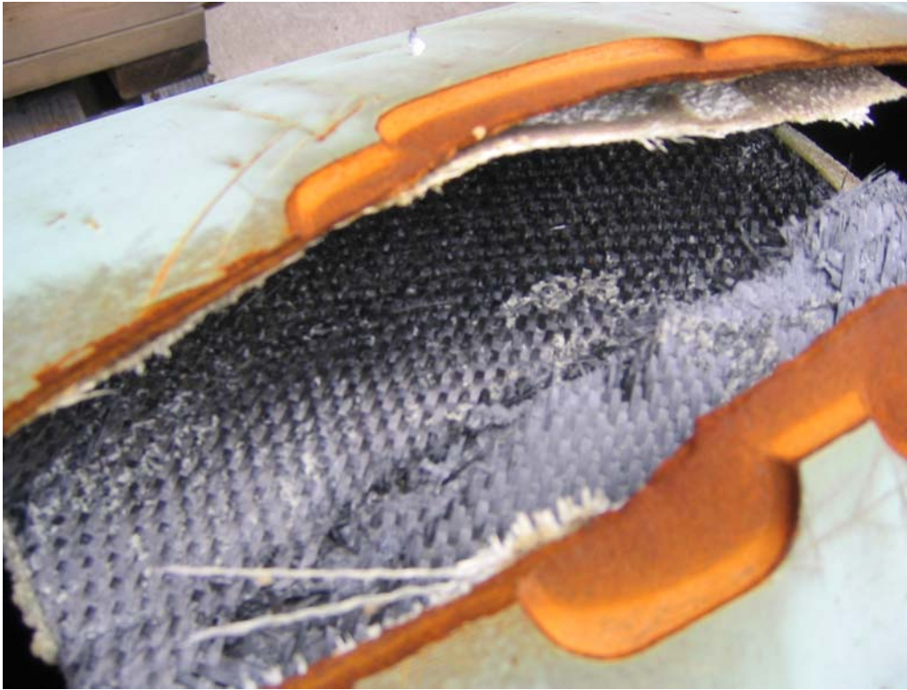
Figure 92 - Magnification of Carbon Fiber-Reinforced Patch After Burst Test
