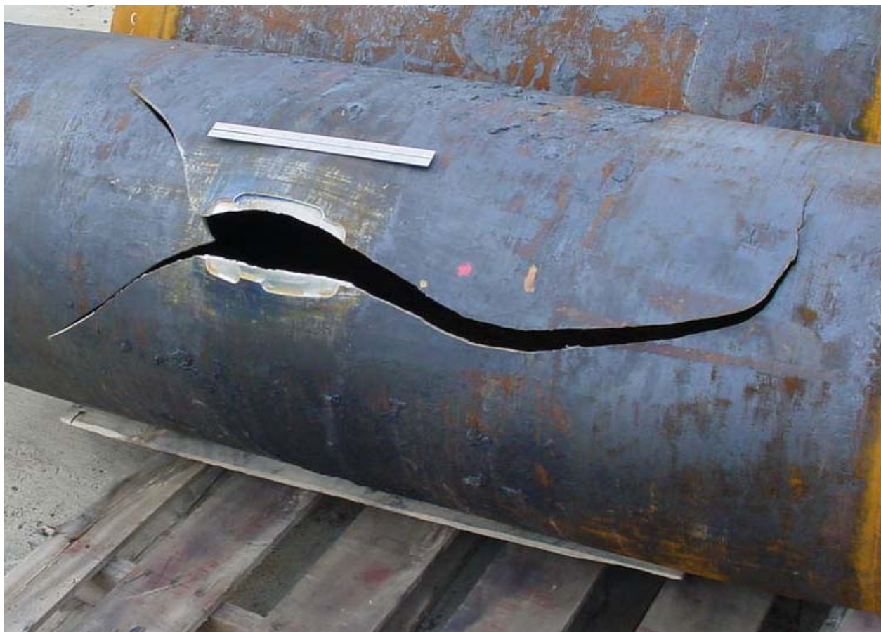
Figure 116 - Hydrostatic Burst Specimen of 558.8 mm (22 in.) With Un-Repaired Damage
