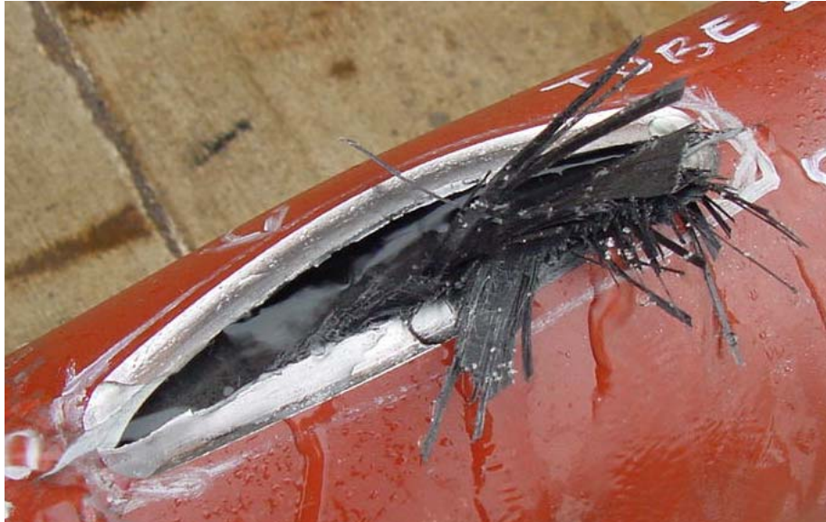
Figure 74 - Pipe Section with Long, Shallow Simulated Corrosion Damage – With Liner – Following Hydrostatic Pressure Test
