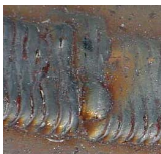
7:00 – Bad Appearance Due Robot Program Error
