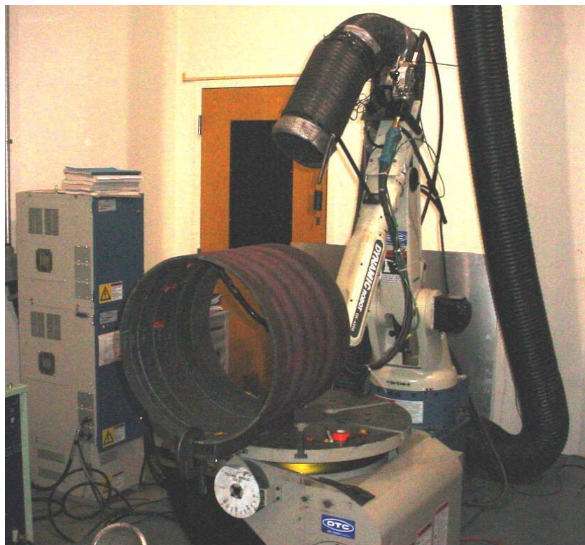
Figure 32 - OTC Robot Set-Up for Internal Welding
