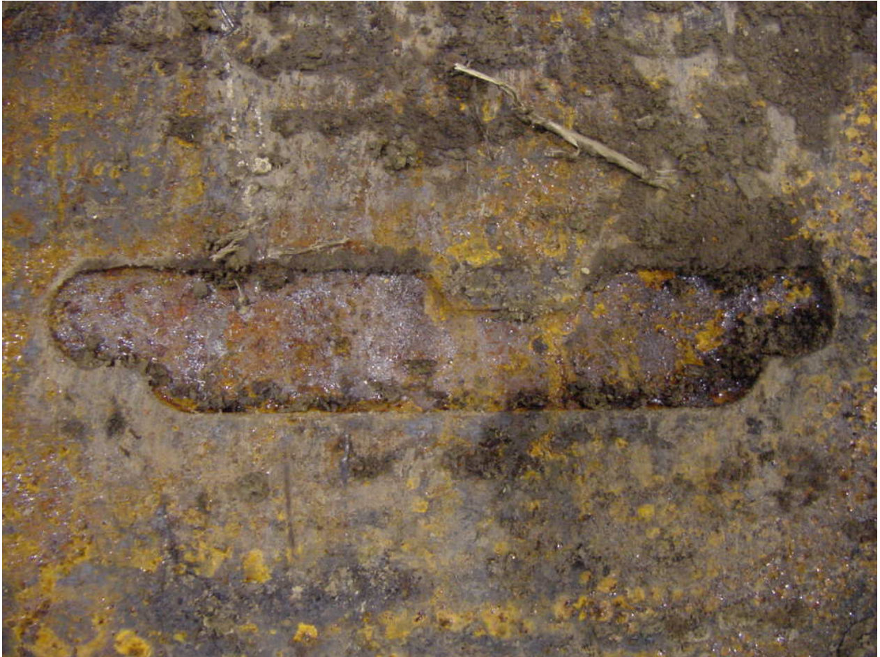
Figure 94 - Simulated Corrosion on Outside of Pipe After Internal Weld Deposition Repair
