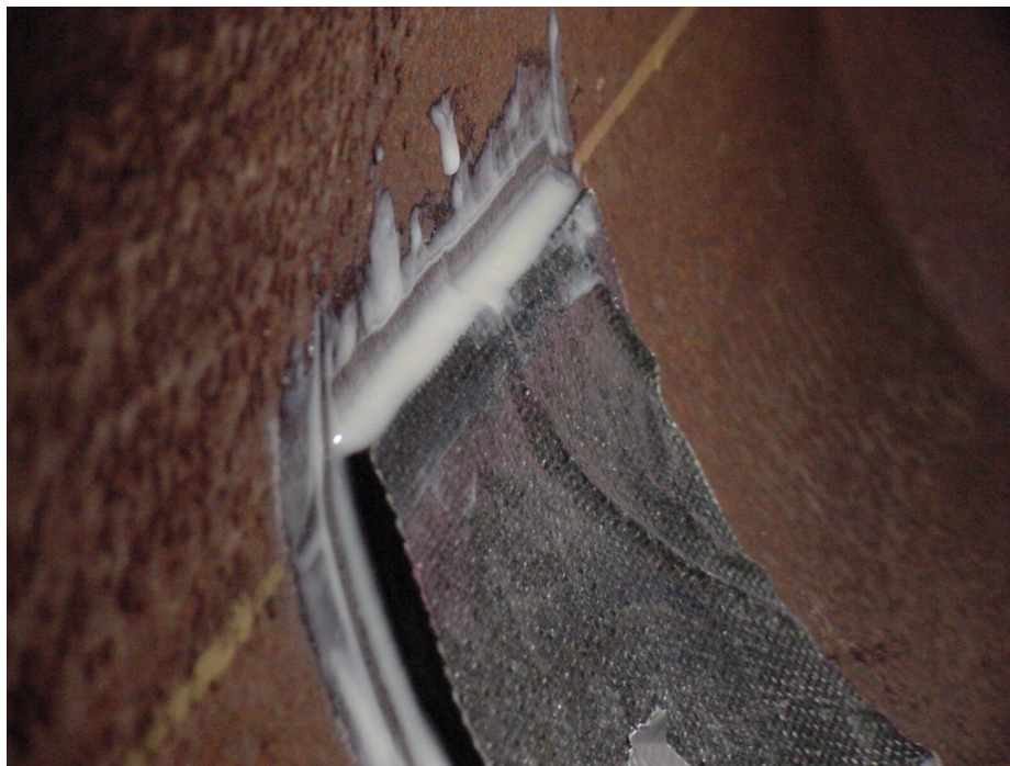
Figure 27 - Adhesive Fillet Around Repair Patch
