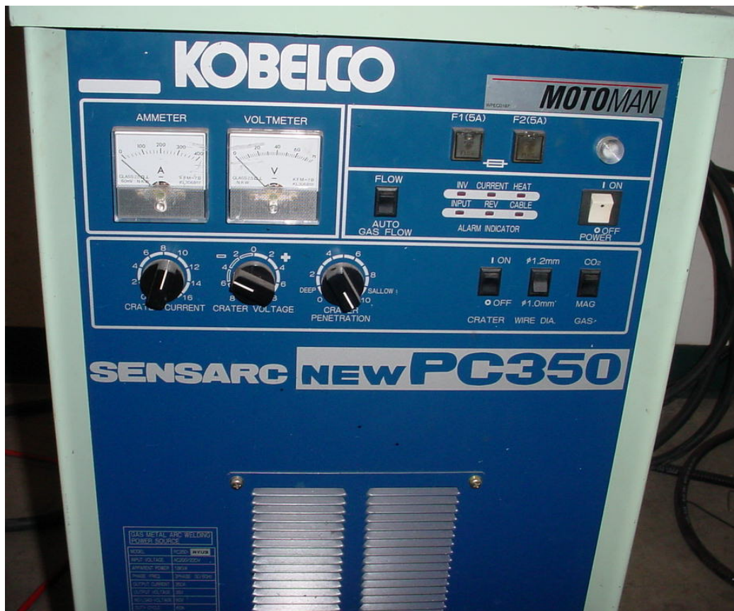
Figure 34 - Kobelco PC-350 Variable Polarity Fuzzy Logic Power Supply
