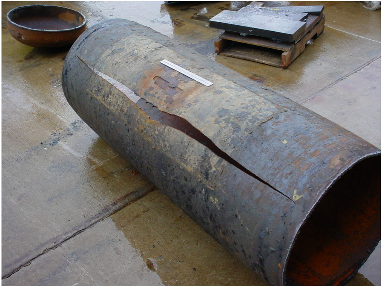
Figure 98 - Pipe Section with Internal Weld Deposition Repair After Hydrostatic Burst Test
