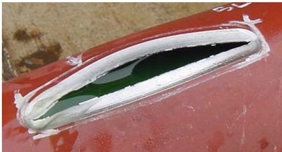
Figure 73 - Pipe Section with Long, Shallow Simulated Corrosion Damage – Without Liner - Following Hydrostatic Pressure Test
