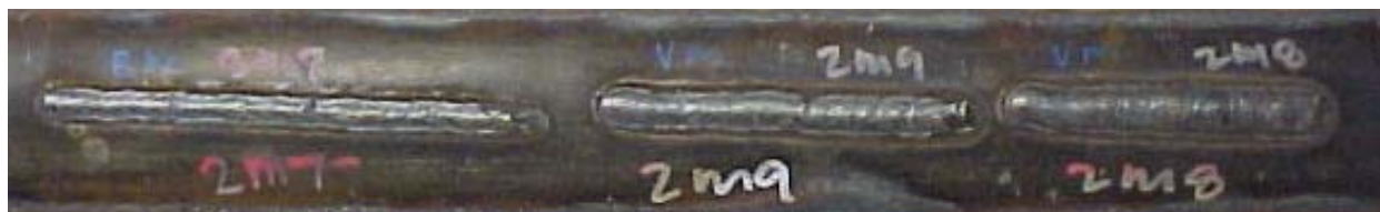
Figure 100 - External Appearance of Welds Made on 3.2 mm (0.125 in.) Thick Pipe with Methane Gas at 4.5 mPa (650 psi) and 6.1 m/sec (19.9 ft/sec) Flow Rate
