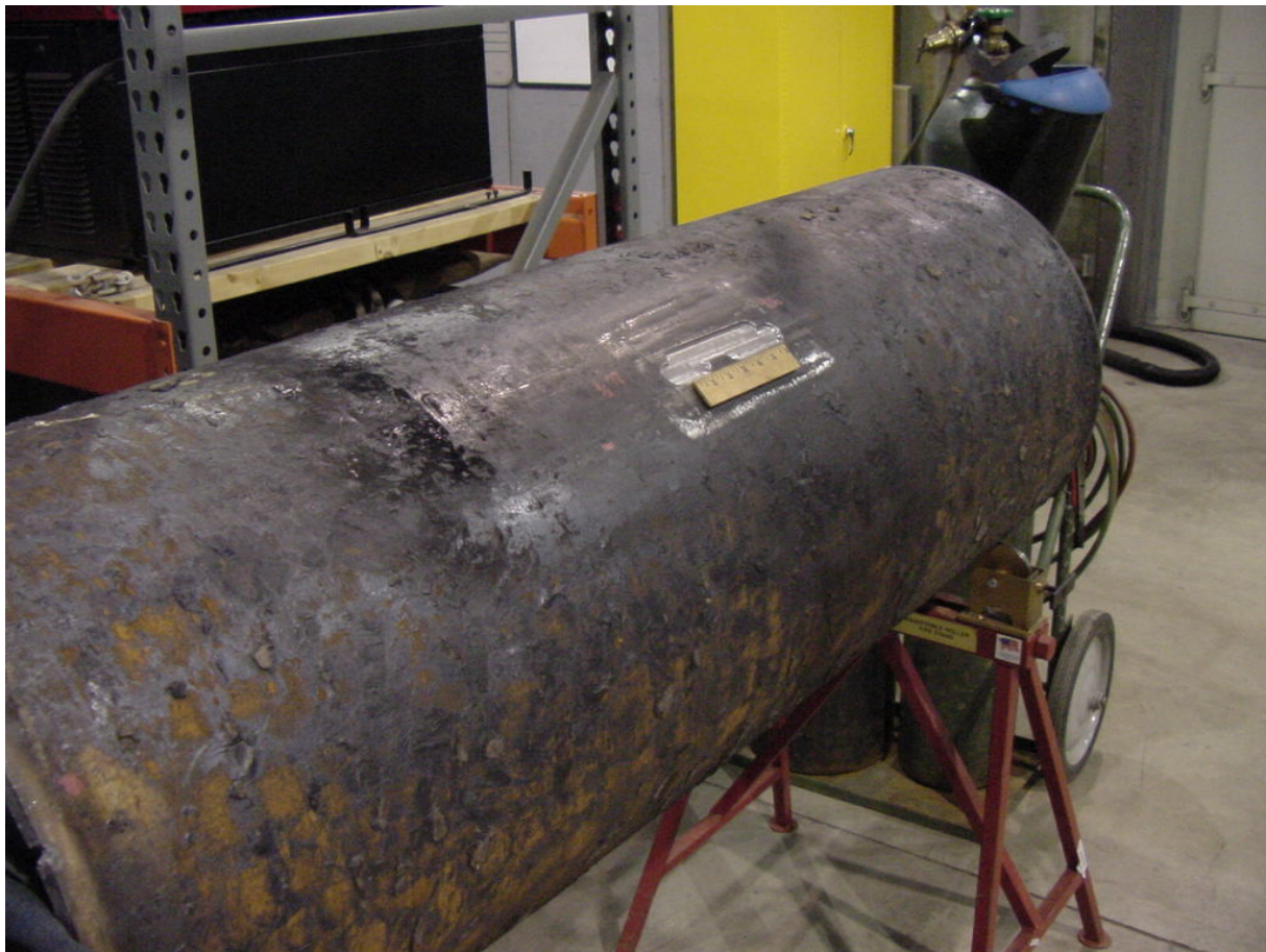
Figure 40 - Simulated Corrosion on 558.80 mm (22 in.) Pipe
