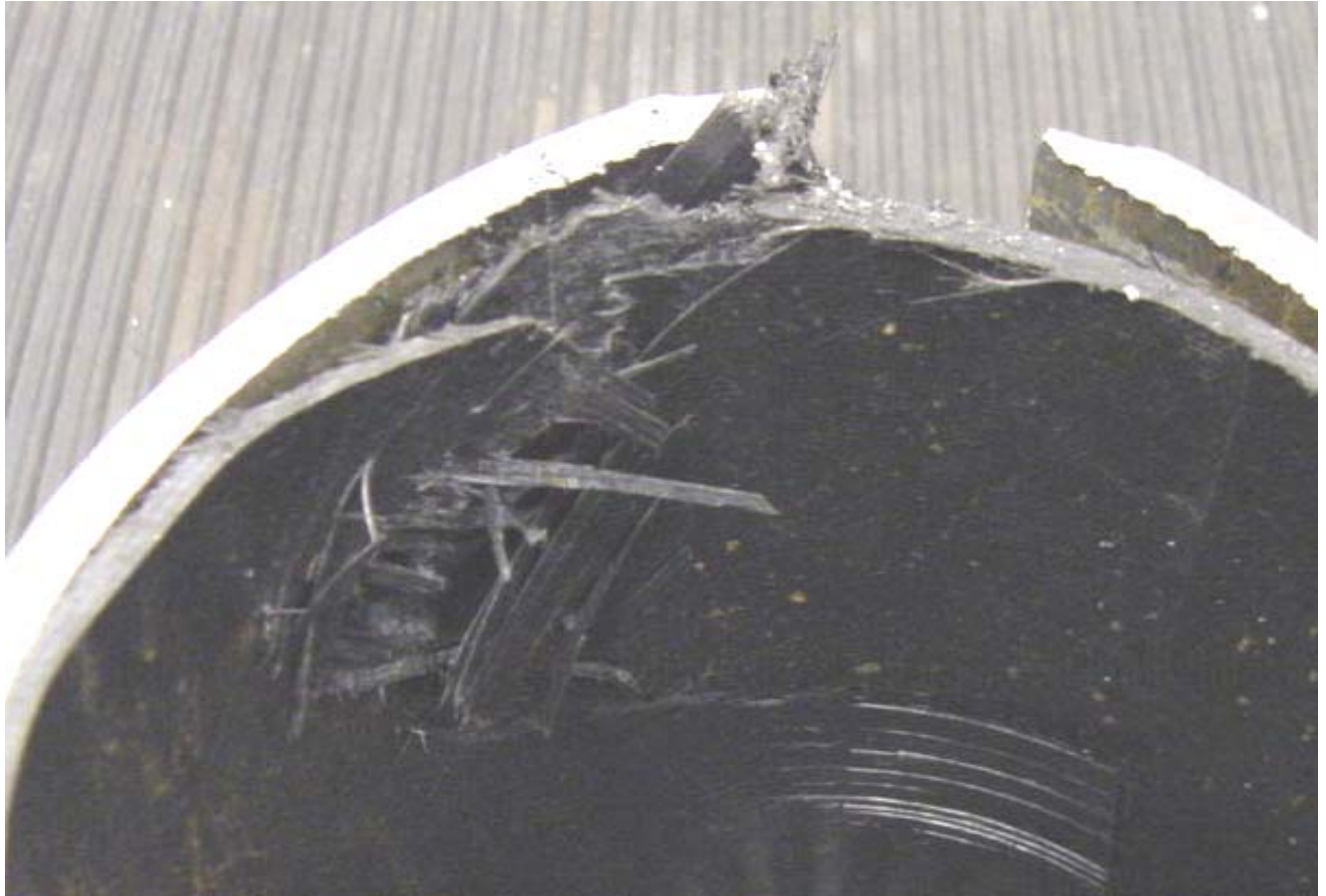
Figure 78 - Pipe Sample Containing Round-Bottom Longitudinal Slot Showing Rupture of Liner Material
