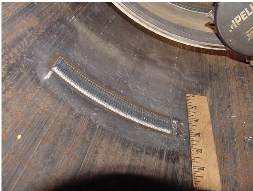
Figure 45 - First Pass of First Layer of Deposited Weld Metal on Inside Pipe Diameter
