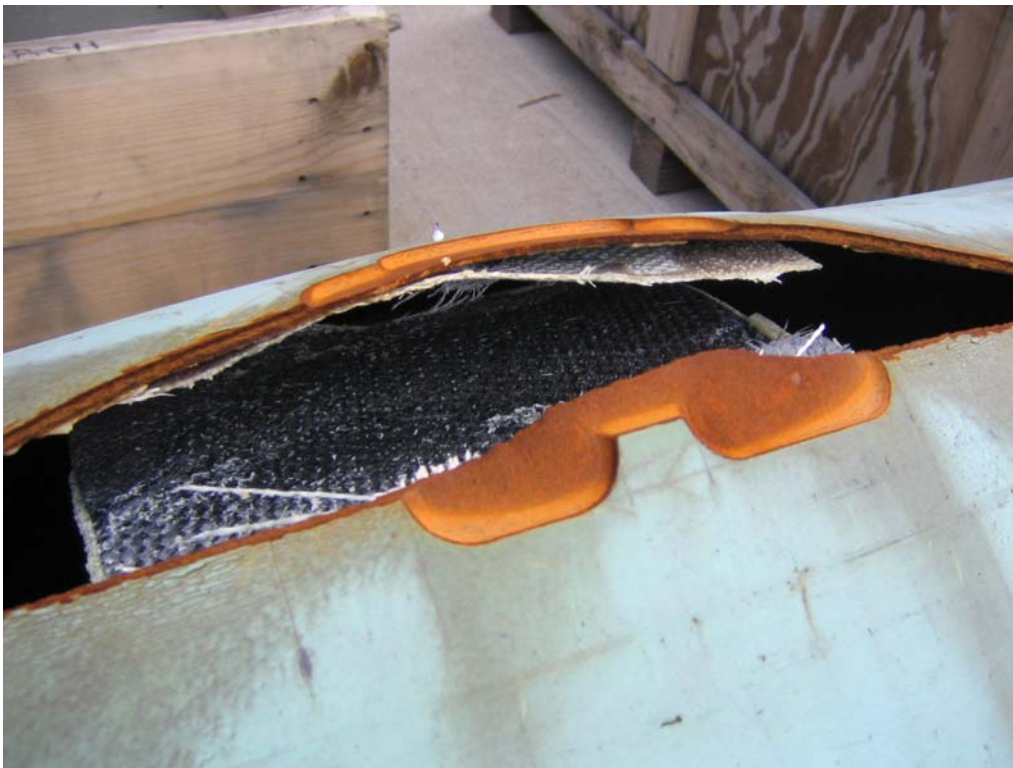
Figure 91 - Failure Initiation Site For Burst Tested Pipe With Carbon Fiber-Reinforced Liner Repair
