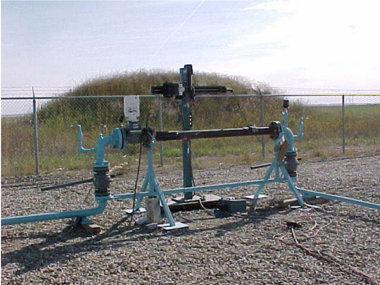
Figure 99 - Experimental Set-Up for Welding onto Thin-Wall Pipe containing Pressurized Methane Gas
