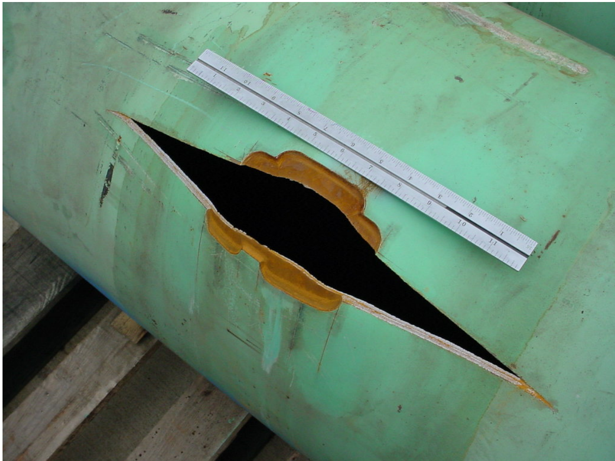
Figure 114 - Hydrostatic Burst Specimen of 508.0 mm (20 in.) with Un-Repaired Damage
