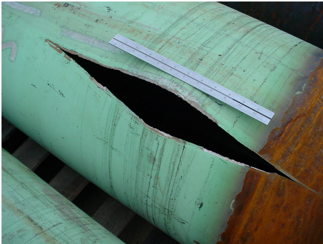
Figure 113 - Hydrostatic Burst Specimen of 508.0 mm (20 in.) in Virgin Pipe
