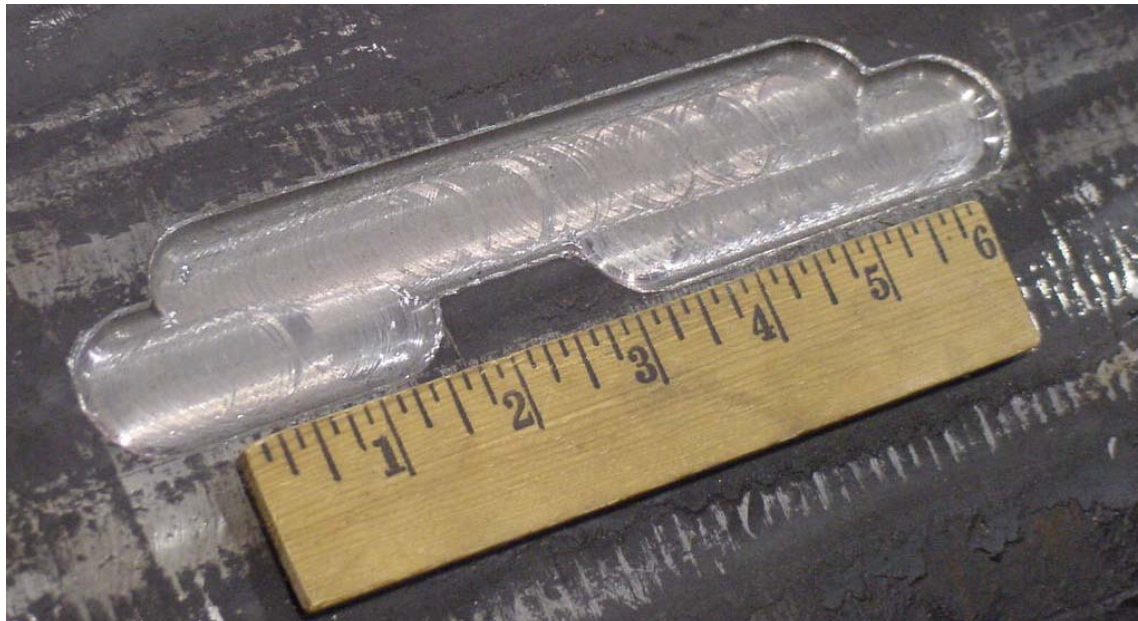
Figure 41 - Magnified View of Simulated Corrosion on 558.80 mm (22 in.) Pipe
