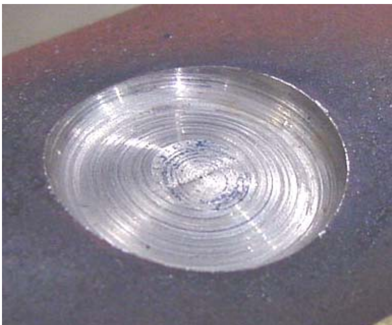
Figure 76 - Pipe Section with Short, Deep Simulated Corrosion Damage – With Liner – Following Hydrostatic Pressure Test
