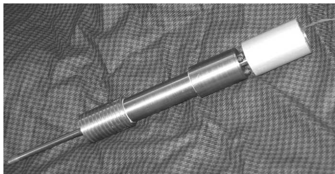
Fig. II.1.5 Double-shaft MR damper made from low-carbon steel
