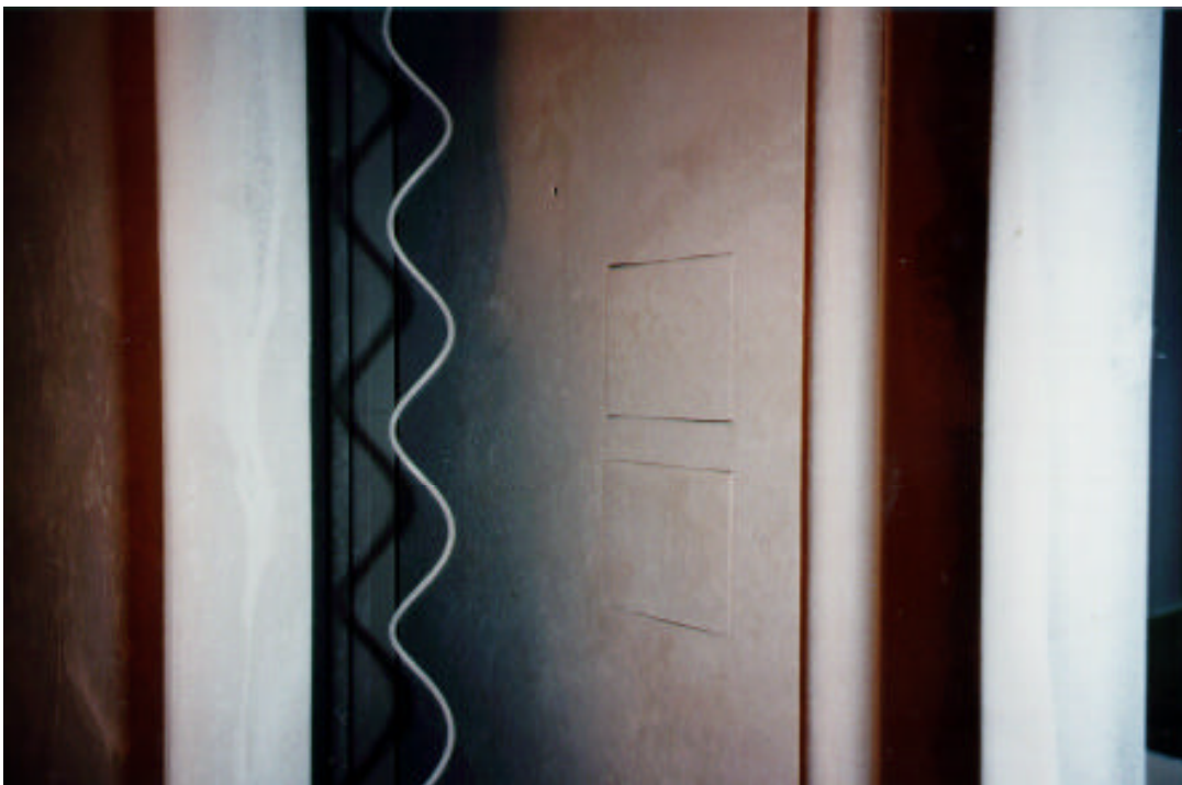
Figure 3.1-4 Pilot ESP Removable Dust Cake Sampling Panels
