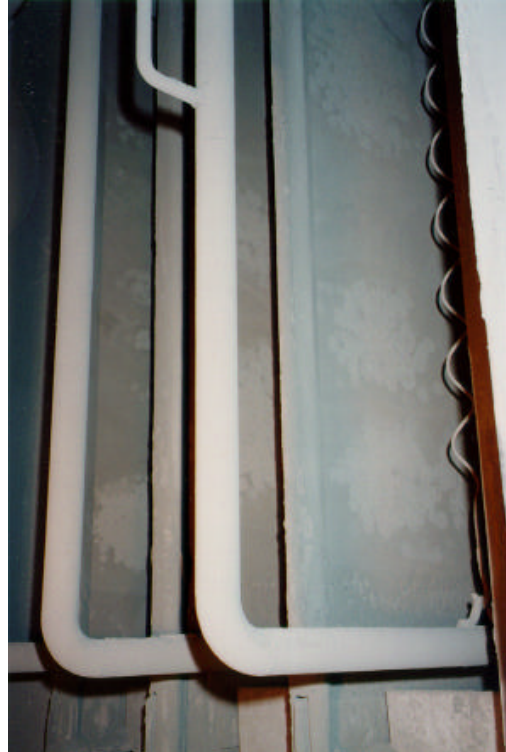
Figure 3.1-3 Pilot ESP Discharge Electrode and Collection Plate Assemblies
