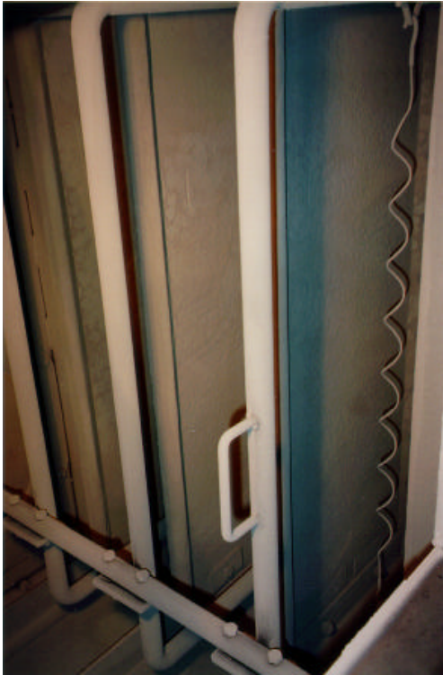
Figure 3.1-3 Pilot ESP Discharge Electrode and Collection Plate Assemblies
