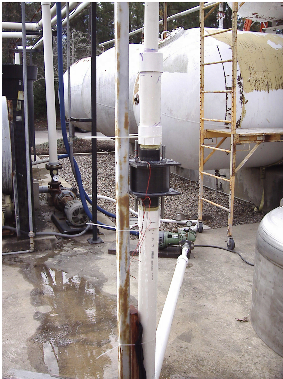
Figure 1 shows the downhole power generator (dark module) in line with flow pipe
