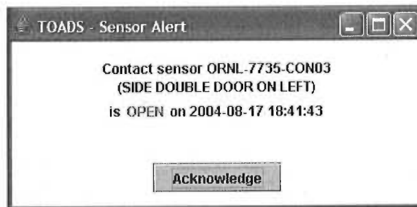
Figure 16. TOADS Alert Screen – An Example of an Open-Door Sensor Alert.
