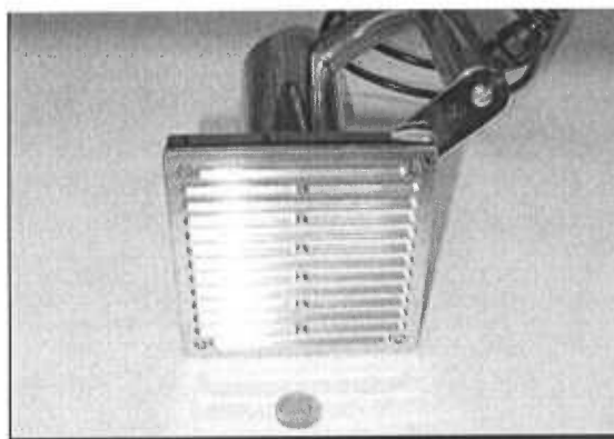
Figure 26. ZnS(Ag) sensor with a 100 cm 2 surface area.
